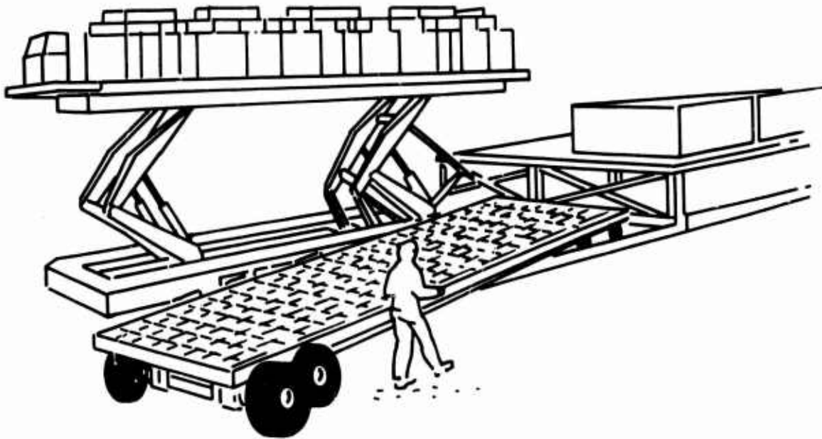
Figure 4. K-loader preparing to interface with another cargo handling system in order to transfer its load
