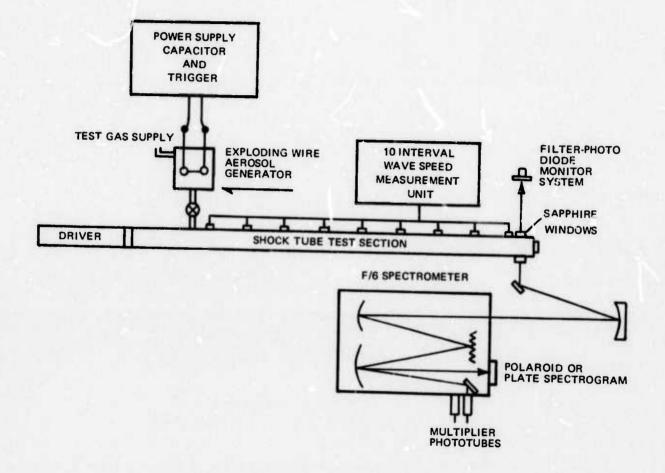
Figure 1 SCHEMATIC DIAGRAM OF EXPERIMENTAL APPARATUS FOR THE MEASUREMENT OF METAL OXIDE SPECTRA. (INSTRUMENTATION SPECIFIC TO THE URANIUM-OXYGEN STUDIES IS DESCRIBED IN THE TEXT.)
