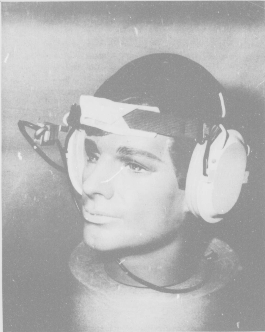
Figure 4 Front view of Communication Headset: light package for O 2 Sensing-Warning System is shown at left; strap across forehead includes sweatband.
