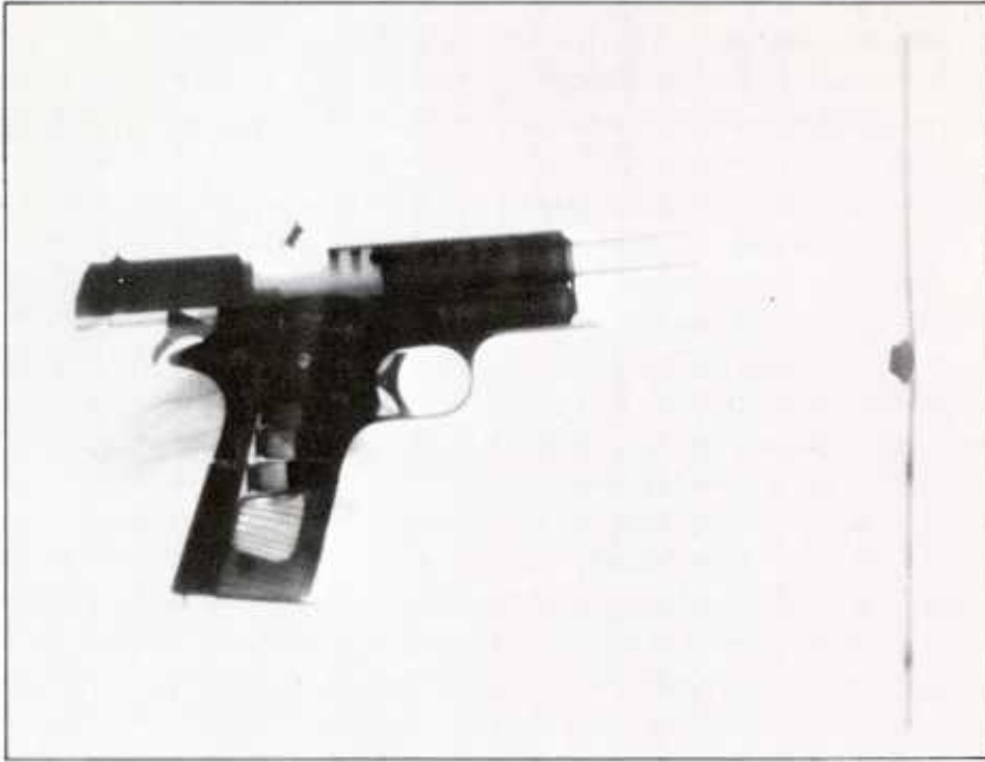
Figure 3. Stop action effect of flash x-ray beam. All motions of a hand held .45-caliber automatic pistol are stopped 12 msec after firing. The shell casing ejects from the chamber as the weapon recoils upward. The lead bullet is seen at right undergoing impact deformation.
