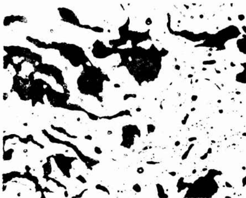
Figure 22. 75 w/o Hastelloy X-ZrO 2 material after exposure for 10 hrs at 2200°F in an inert environment followed by exposure to a dynamic oxidizing environment for 16 hours at 2125°F.
