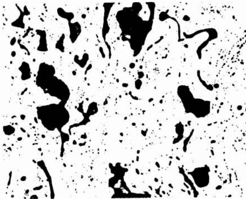
Figure 21. 75 w/o Hastelloy X-ZrO 2 material after exposure for 10 hrs at 2200°F in an inert environment followed by exposure to a dynamic oxidizing environment for 7 hours at 2125°F.
