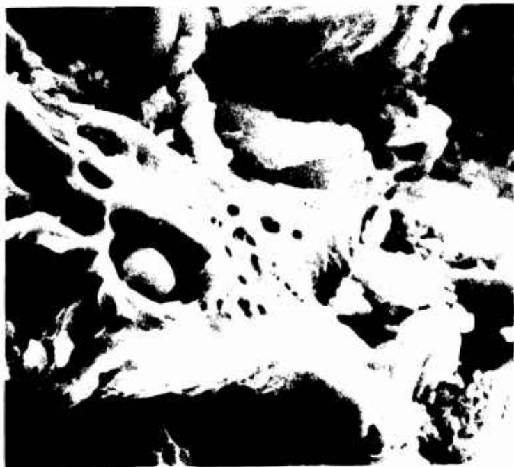
Figure 38. Fracture surface of 50 w/o Hastelloy X-ZrO 2 (Group A) tensile specimen which had been exposed for 100 hours at 2200°F in an inert environment. Ductile tensile fracture of the Hastelloy X phase is clearly shown in these fractographs.
