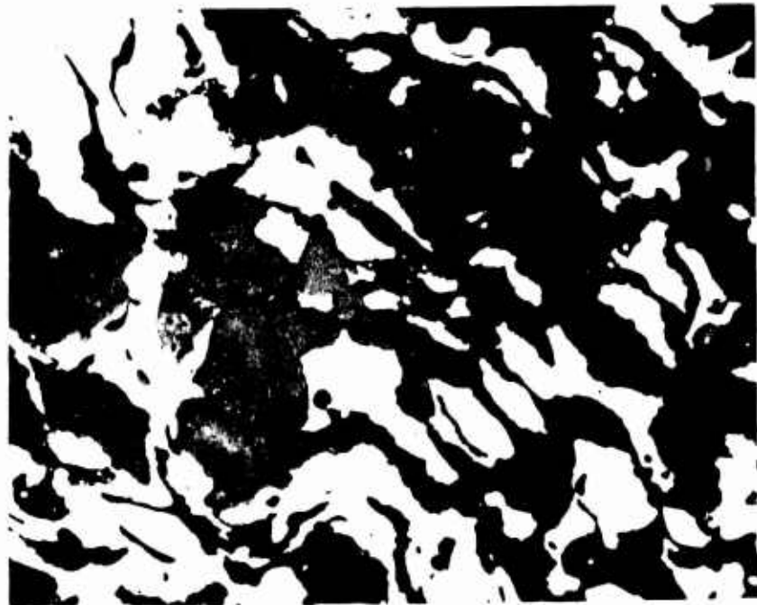
Figure 14. 50 w/o Hastelloy X-ZrO 2 (Group B) material after exposure for 100 hours at 2200°F in an inert environment.
