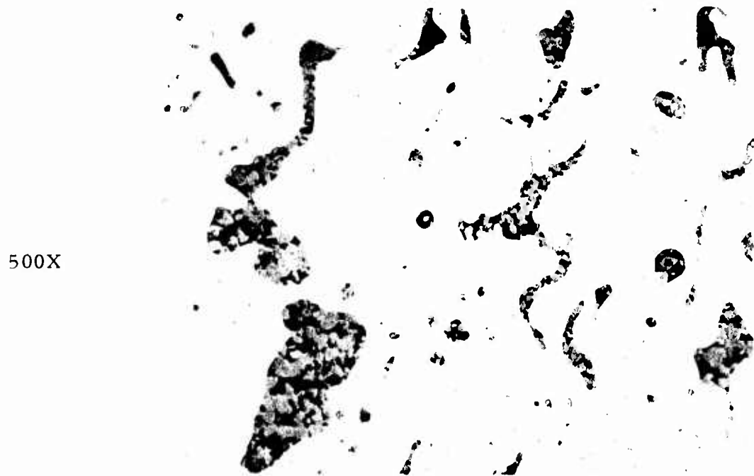
Figure 20. 75 w/o Hastelloy X-ZrO 2 material after exposure for 100 hrs at 2200°F in an inert environment. The same characteristics found in the 10 hour exposed material are seen here. No changes in distribution or character of the material from the 10 hour exposure are apparent.
