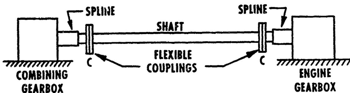
Figure 15. Schematic of Typical Cross Shaft Assembly.
