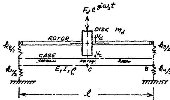
Figure 22. Simplified Model of Engine Case/Rotor Assembly.
