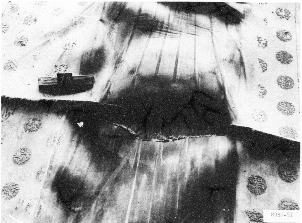
Photo 20. Failure of run 3 of XW18 membrane section 1
