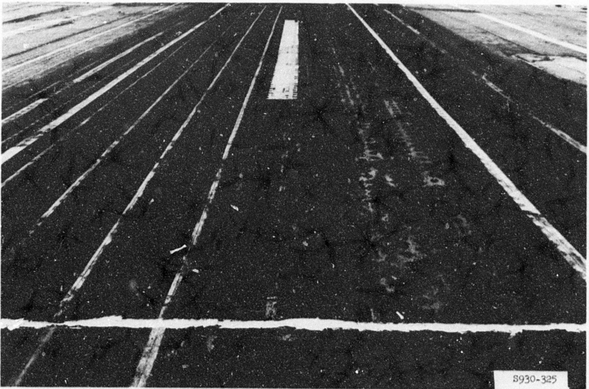
Photo 70. Condition of membrane sheet 2 of test section 1 after 910 coverages
