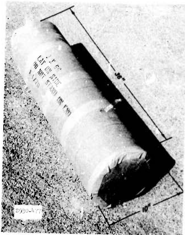
Fig. 1. Roll of XW18 membrane surfacing, 3 ft wide and 66 ft long
