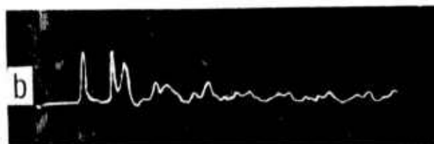
Figure 10. Interferometer Output Obtained by Firing the Pulsed Phase Shifter in the Short-Pulse Laser Cavity Shown in Figure 9.
