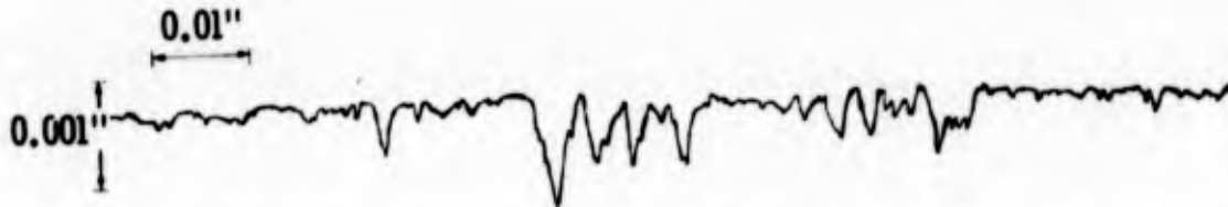
(c) SPECIMEN #348 LIGHT PITTING (1.2 MM DROPS, APPROX. 2000 FT/SEC) (TREATED MATERIAL)
