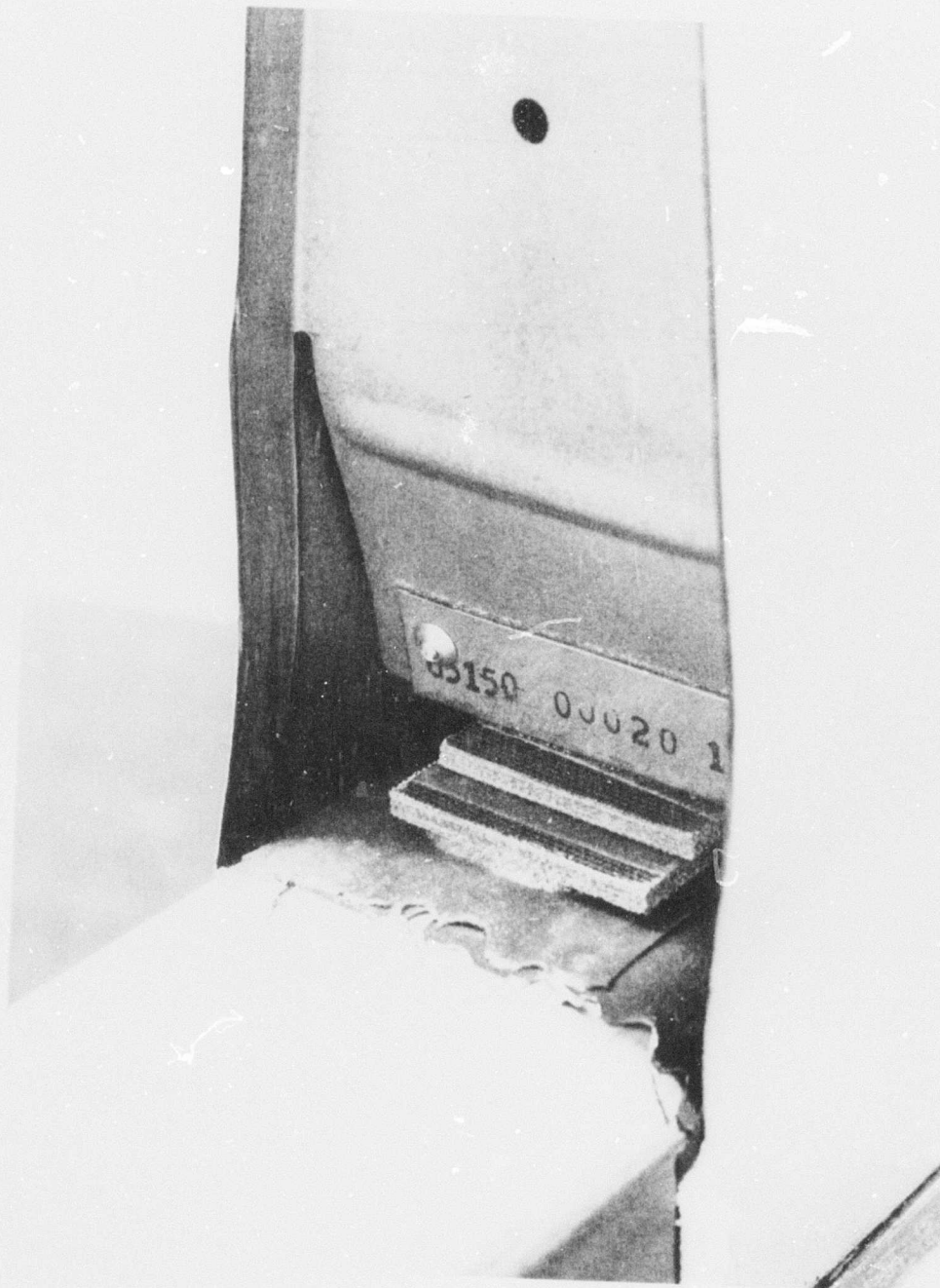
Figure 6. Internal Rib Relief Pocket Design Showing Rib Movement During Bonding.
