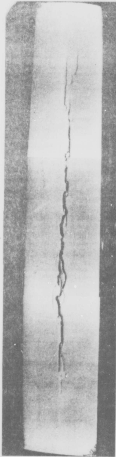
FIGURE 15 POLISHED SECTION THROUGH POLYCARBONATE SPECIMEN NO. 6 SHOWING THE DISTRIBUTION OF CRACKS INTERSECTING THE SURFACE
