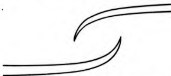
(c) STRESS IS REMOVED AND CRACKS HAVE STOPPED. CRACKS WHICH WERE PENNY-SHAPED IN THEIR EARLY STAGES OF FORMATION ARE NOW DISH-SHAPED.
