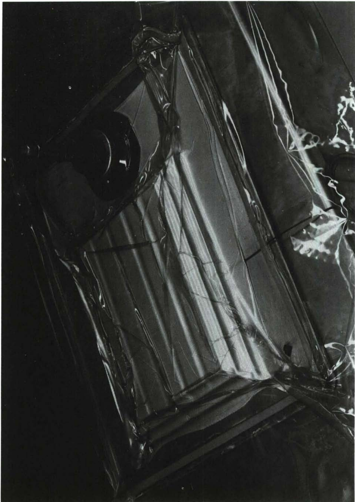
Figure 20: MOLD CAVITY – BAGGED AND VACUUM APPLIED
