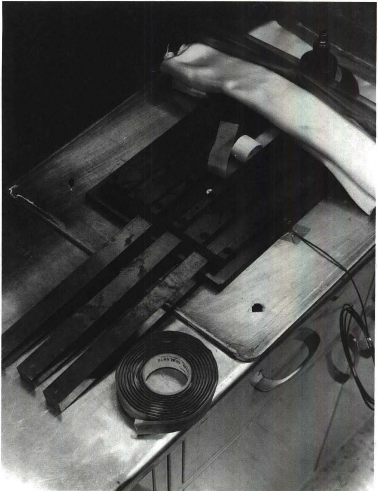
Figure 19: MOLD CAVITY – SPECIMEN INSTALLATION AND BAGGING OPERATION
