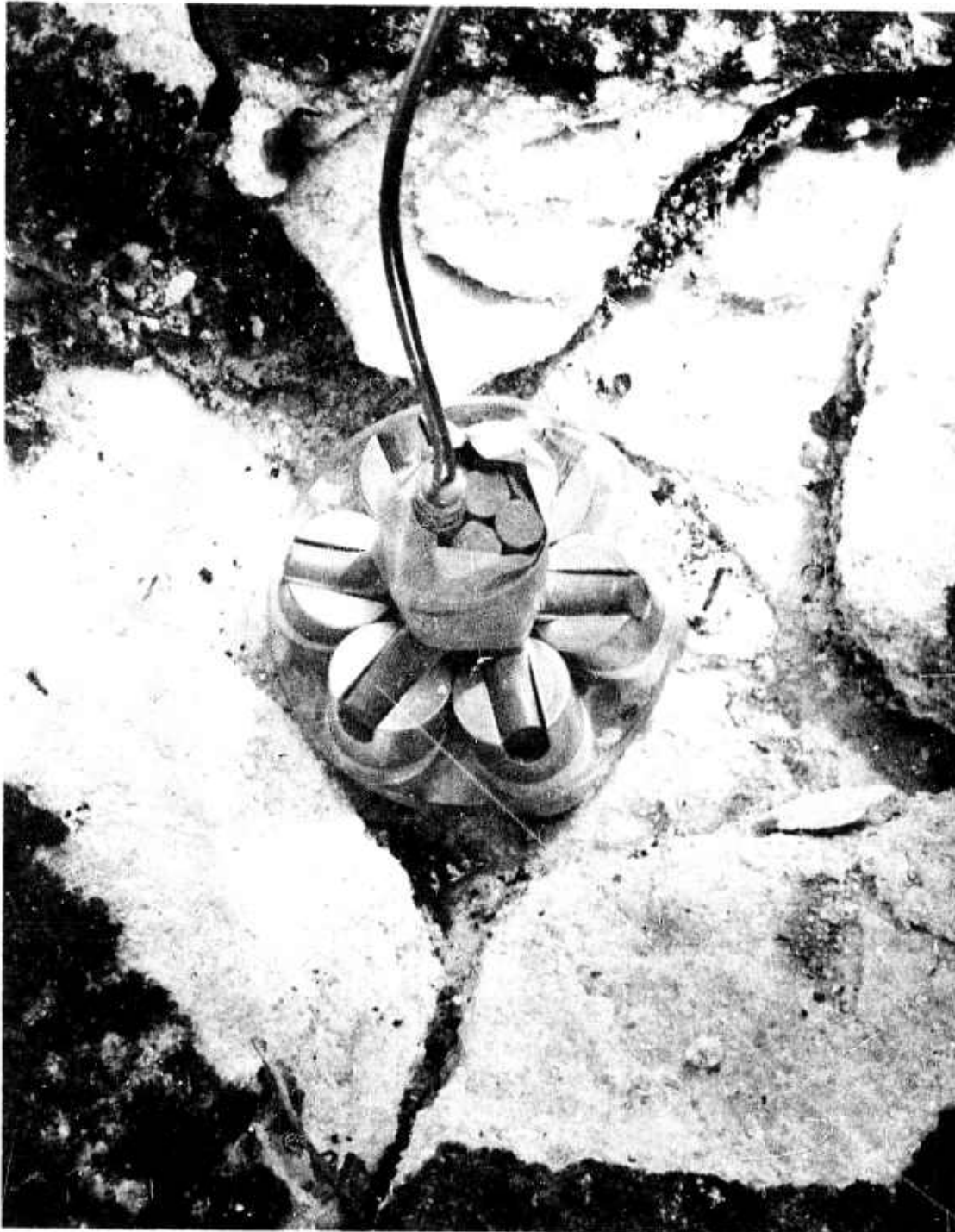
7-Charge Cluster Unit - Emplaced on Rock Prior to Firing
