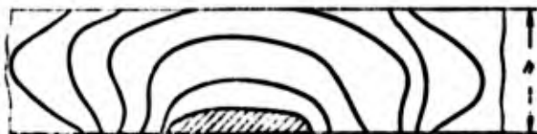
Figure 18. Crack propagation from part-through defect in plane specimen (initial defect shown hatched).
