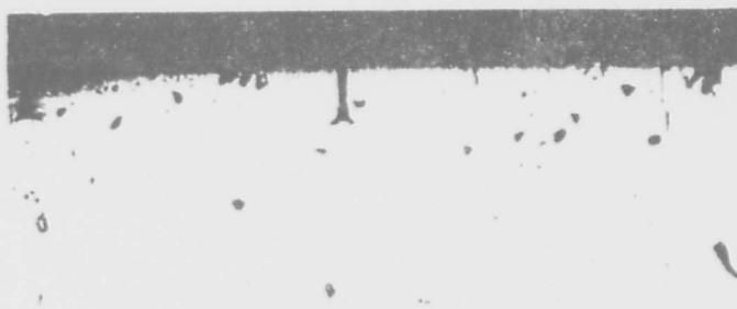
Figure 16. Open cracks with blunt edge in polycarbonate specimen (x 66.5) ( y = 0.96 mm; t = 22 hours; T = 22^\circ C).
