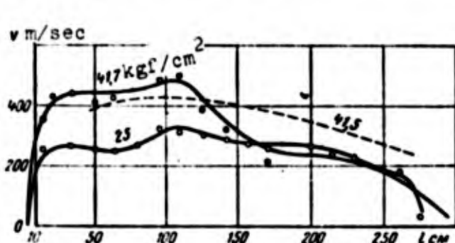
Figure 63. Crack propagation velocity in acrylon specimens with nonuniform nominal stress distribution along specimen edges in accordance with the diagrams of Figure 61 (solid curves).
