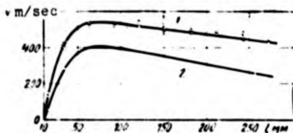
Figure 47. Crack propagation velocity in tests of square acrylon specimens as function of stress level.
