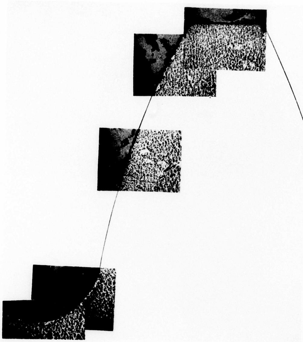
Figure 38. Grain Flow Pattern After Grinding - Roll-Generated Gear.
