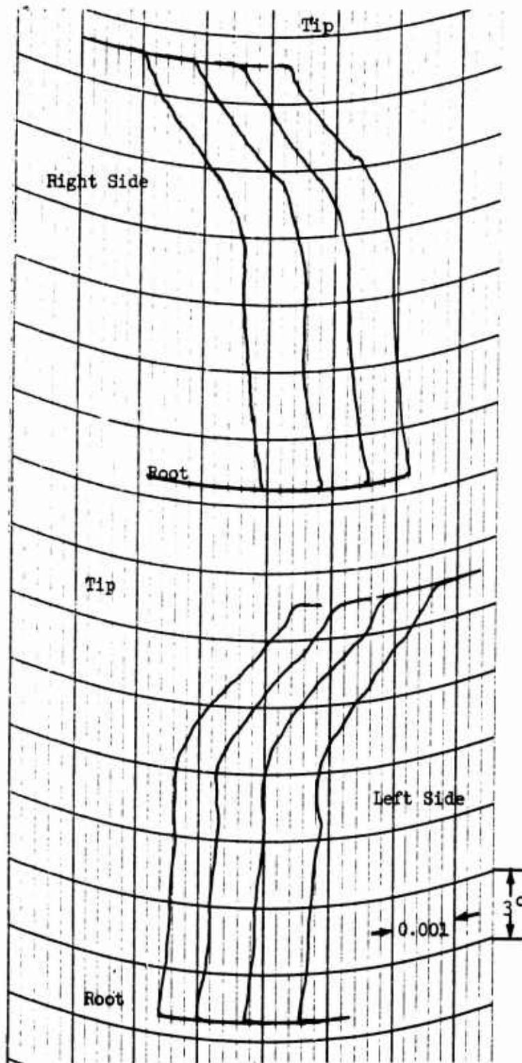
Figure 8. Involute Profile Chart for Finished Test Gear.
