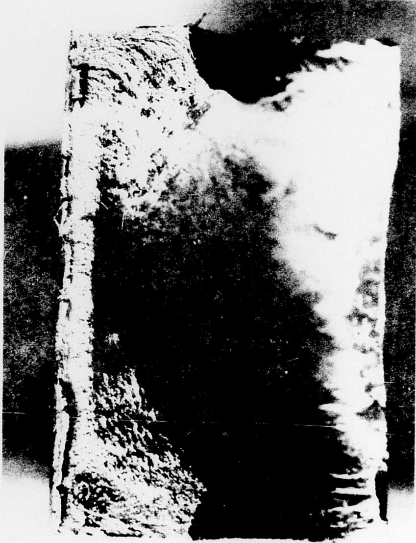
Figure 28. Typical Single-Tooth Static Fracture.
