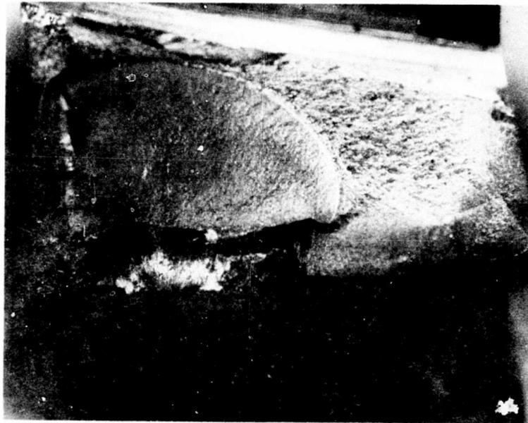
Figure 31. Fatigue Crack Originating From Surface Pit.
