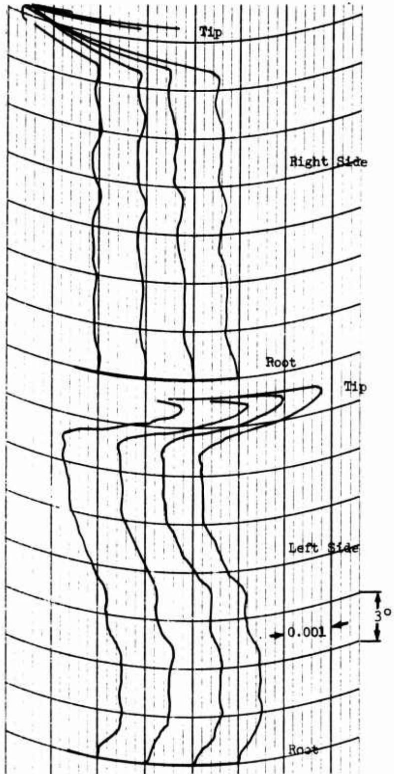
Figure 6. Involute Profile Chart for Roll-Formed Process - As Rolled.
