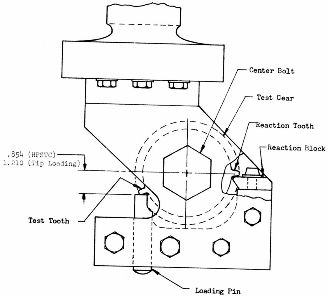
Figure 15. Schematic of Gear Test Fixture.
