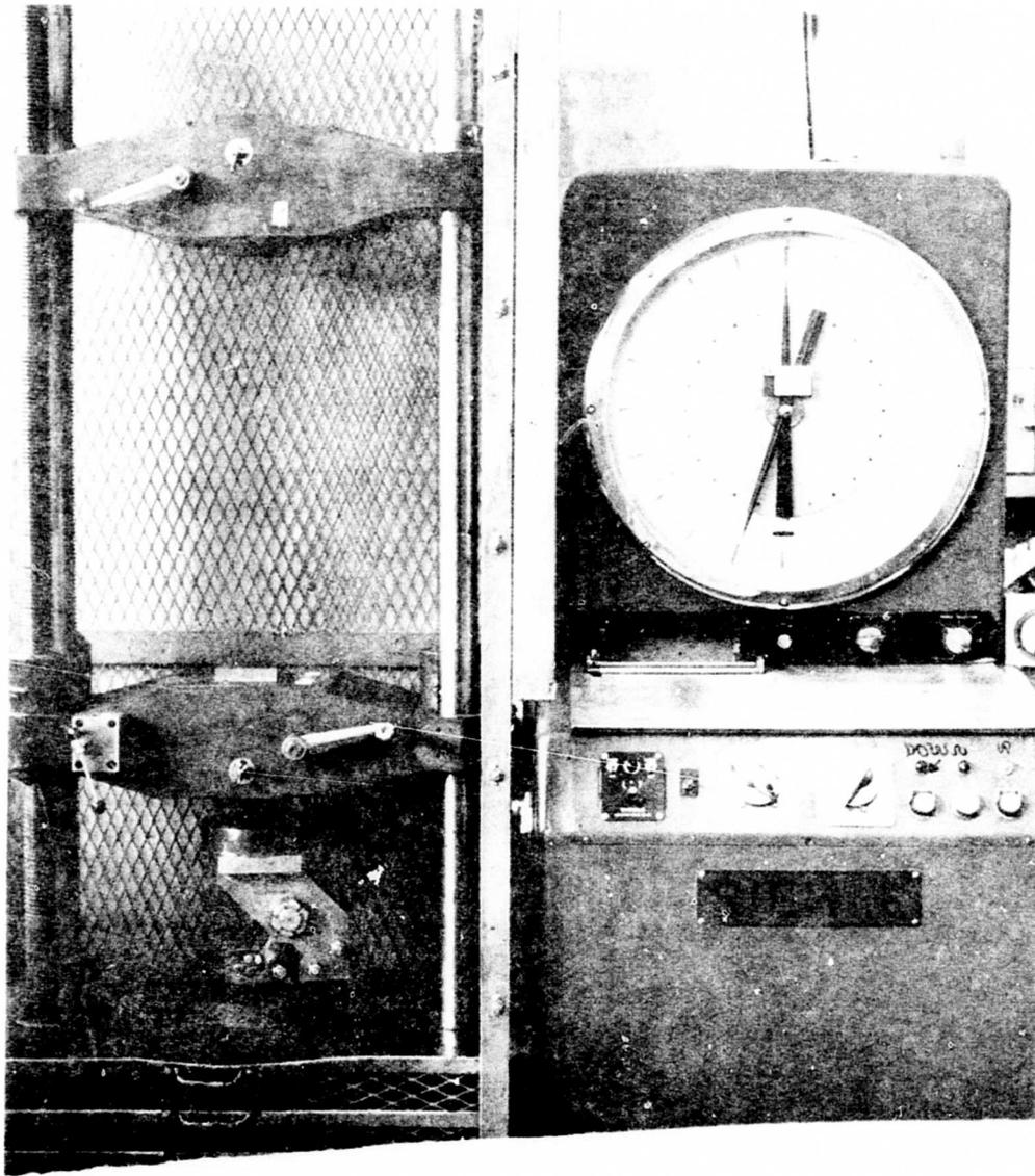
Figure 16. Static Test Arrangement in the Riehle Tensile Machine.
