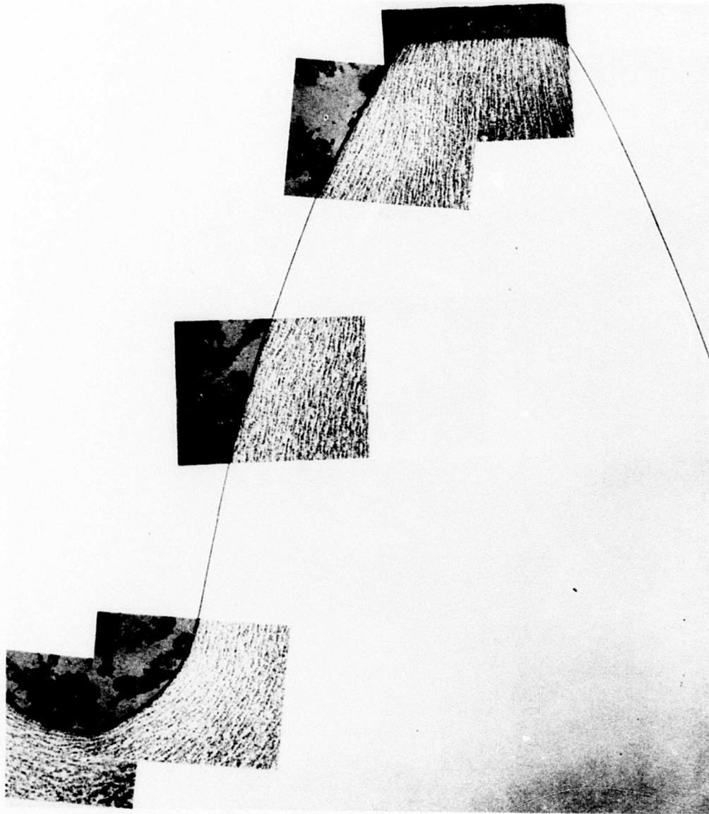
Figure 37. Grain Flow Pattern After Grinding - Roll-Formed Gear.
