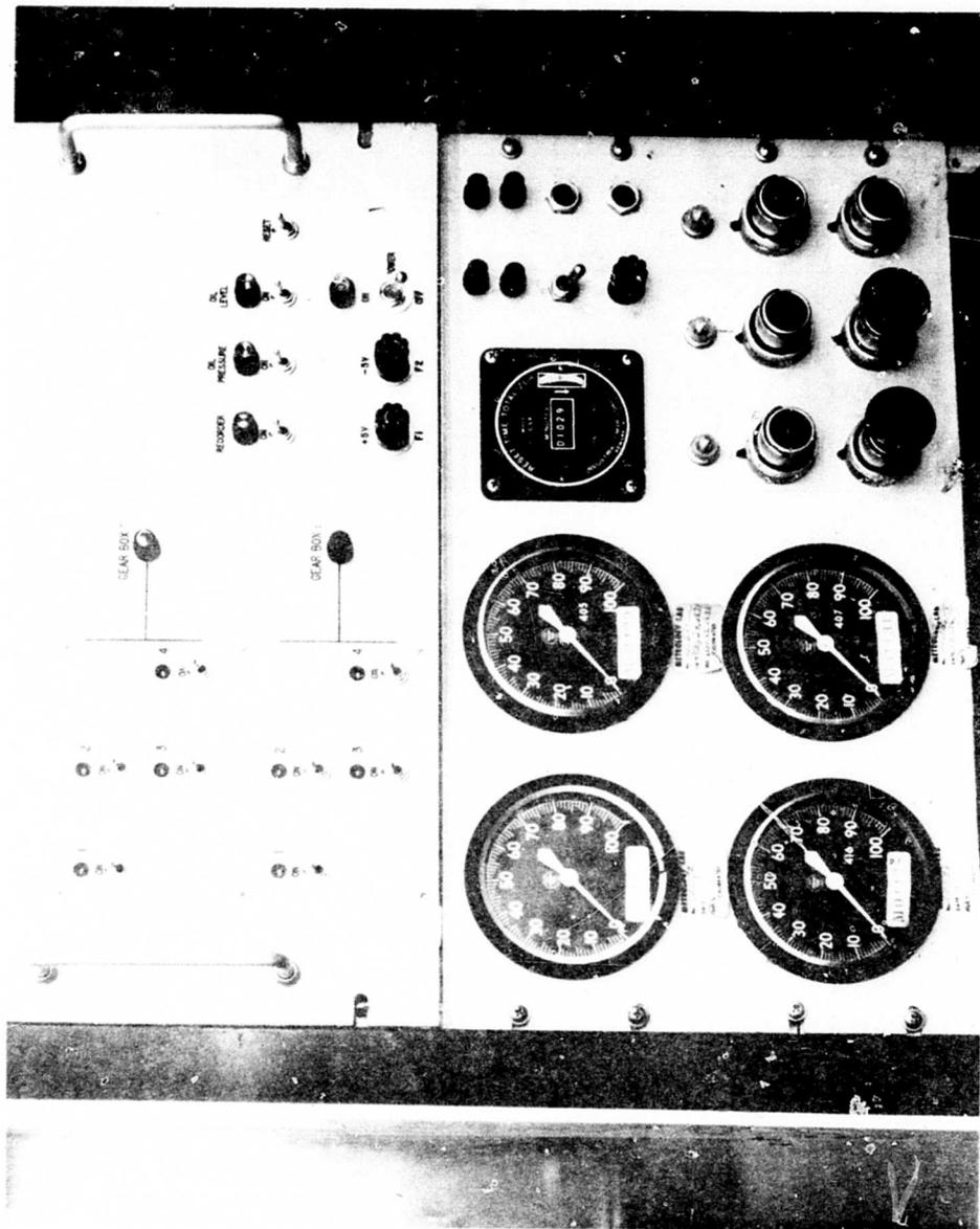
Figure 18. Instrument Panel - Four-Inch Gear Tester.
