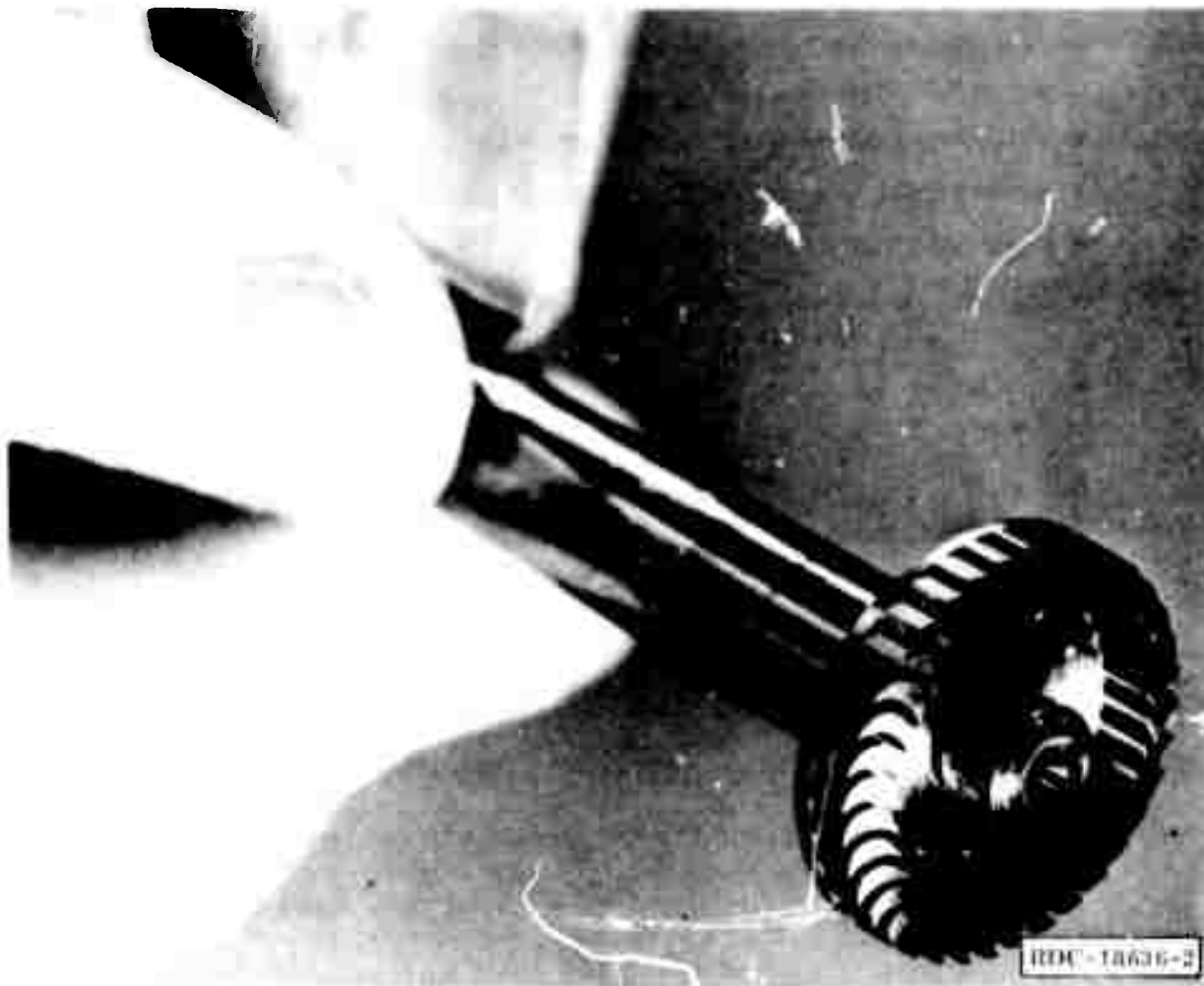
Figure 17. Radial Impulse Turbine Wheel (0.625-Inch-Diameter) Mounted on 0.261-Inch-Diameter Alternator Shaft
