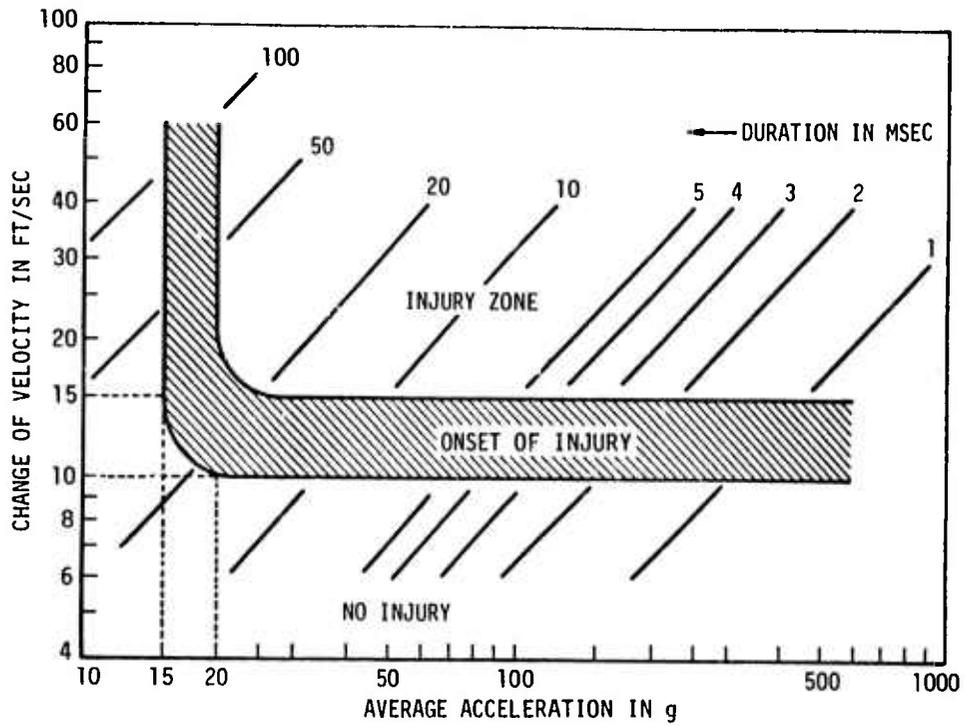
Figure 2 - Tolerance of Man to Short-Duration Shock Motion
