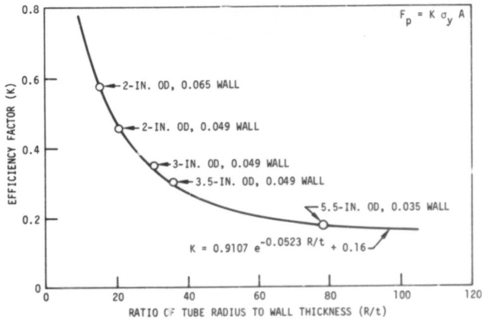
Figure 29 - Experimentally Determined Efficiency Factors, Inextensional Buckling
