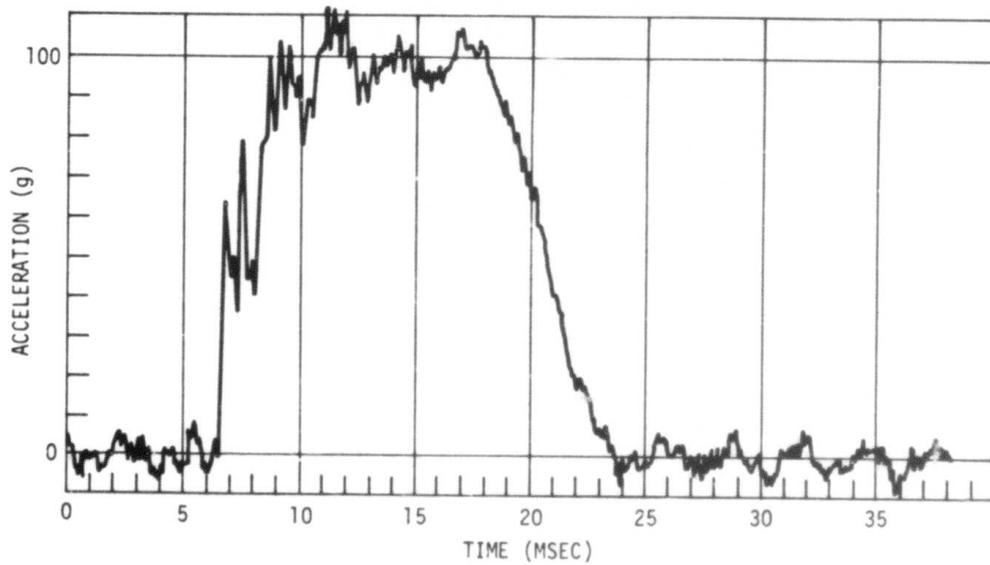
Figure 40 - Experimental Data for Bumper Tube
