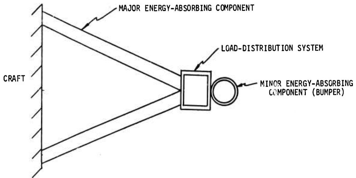
Figure 6 - Possible Configuration of Extremity Structure
