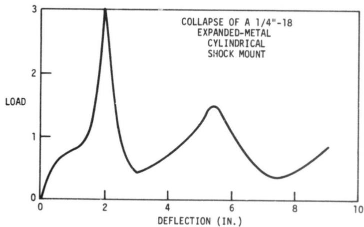
Figure 19 - Load-Deflection Curve for an Expanded-Metal Tube
