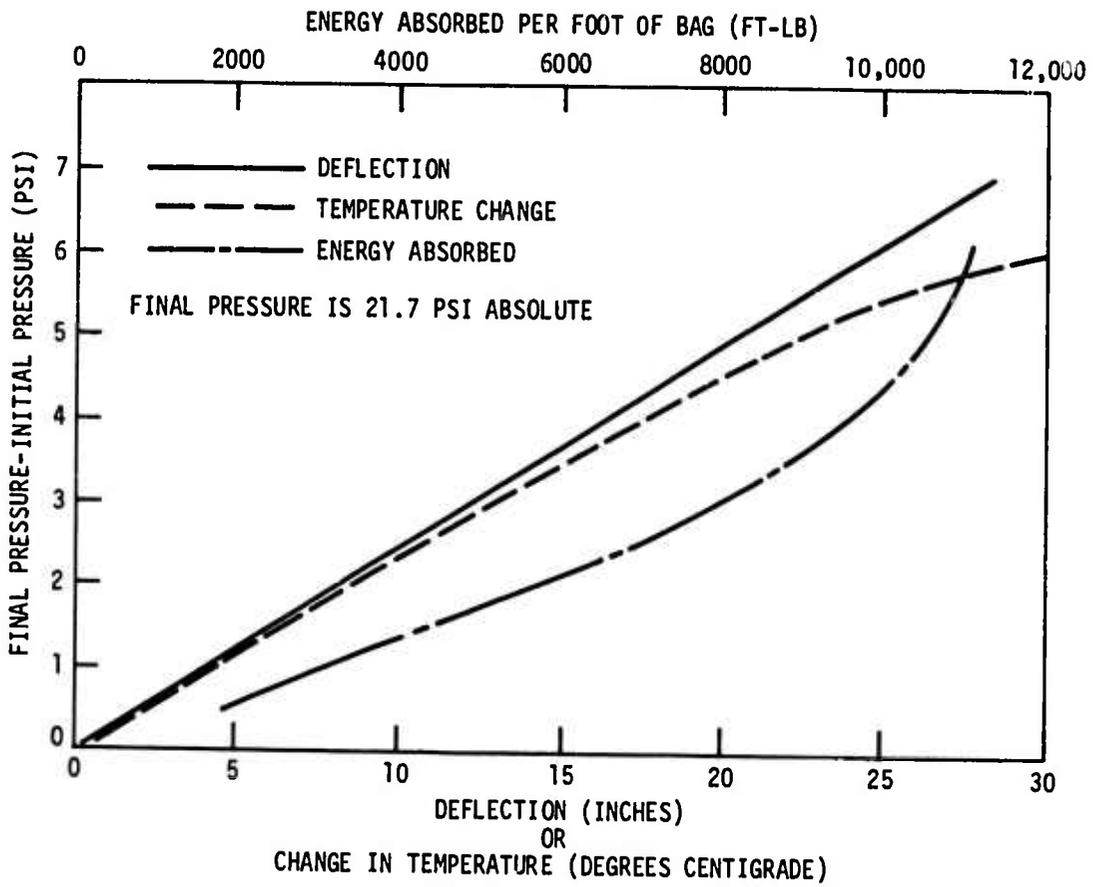
Figure 10 - Adiabatic Compression in a Sample Gas-Filled Bag
