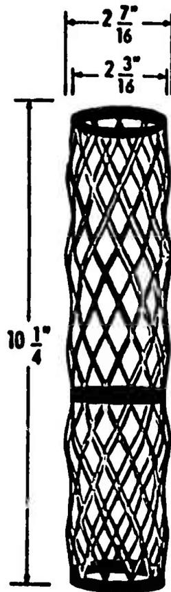
Figure 14 - General Motors Energy-Absorbing Steering Column
