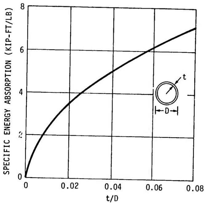
Figure 22 - Specific Energy Absorption for Inverting Tube
