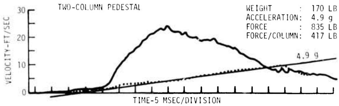
Figure 16 - Experimental Data for Energy-Absorbing Steering Column
