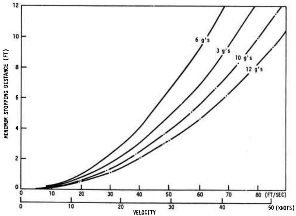
Figure 3 - Minimum Stopping Distance for Critical Acceleration Environment
