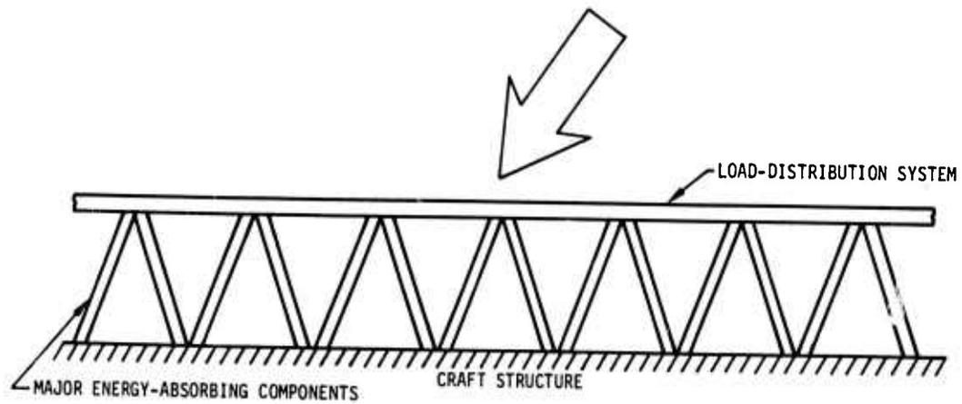
Figure 34 - An Integrated Protection System, Extremity Structure
