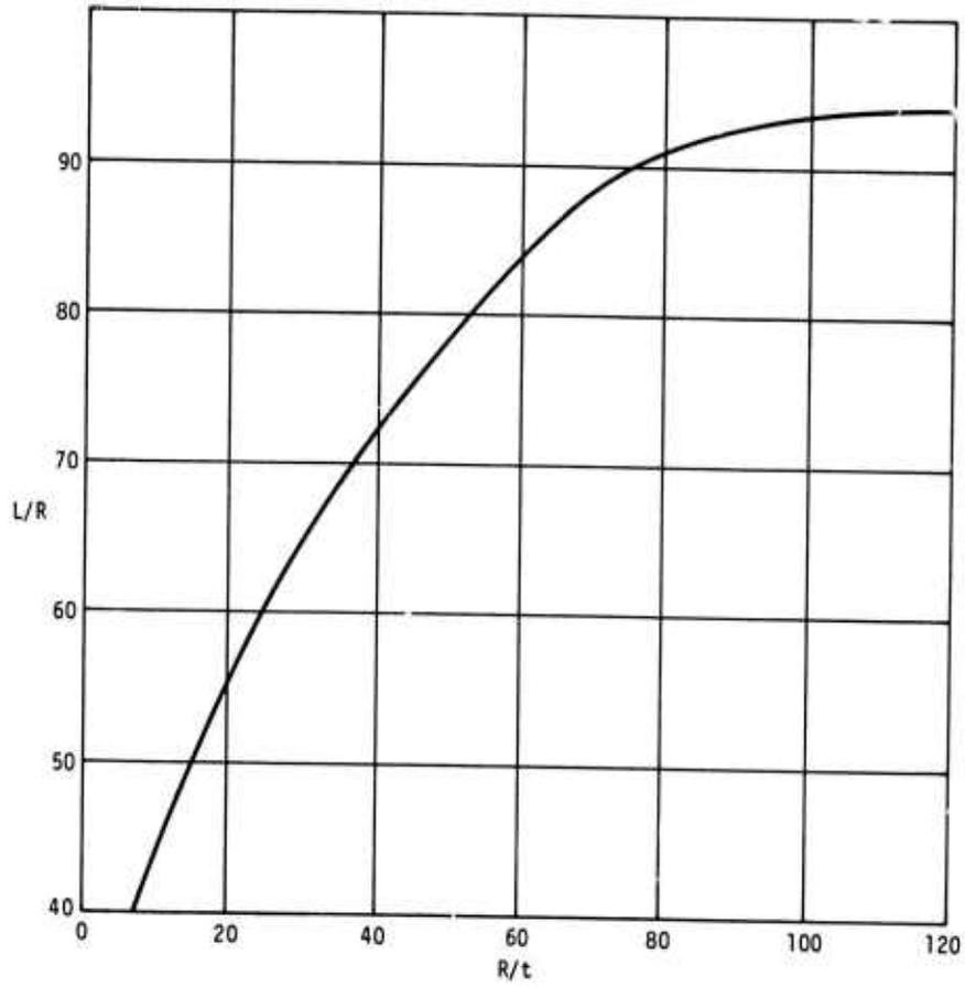
Figure 33 - L/R versus R/t for 6061-T6 Aluminum Tubes
