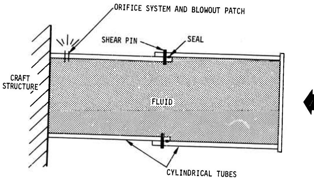
Figure 26 - Fluid Dispersal Shock Absorber
