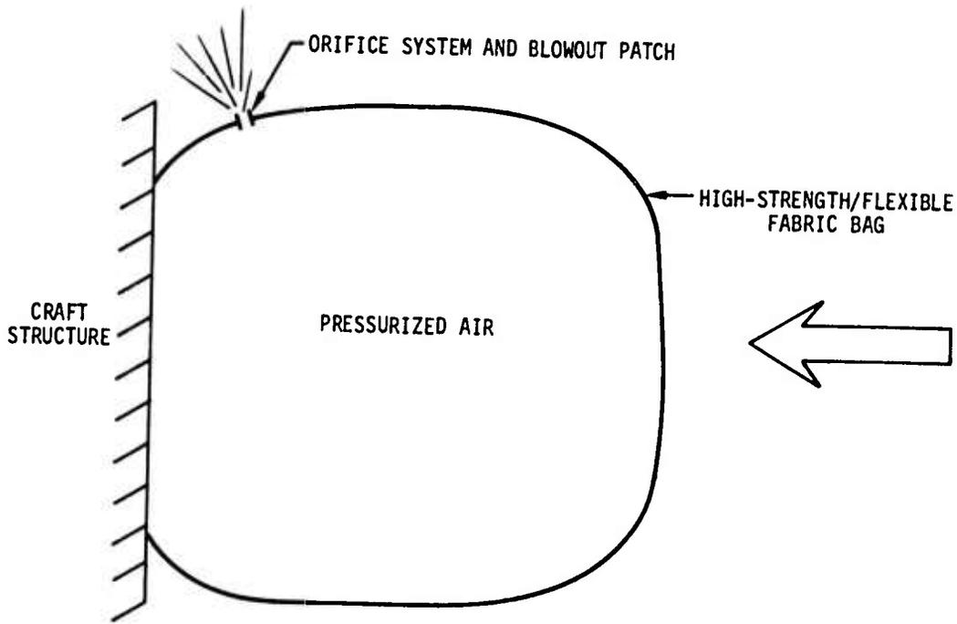
Figure 8 - Air Bag as an Energy Absorber
