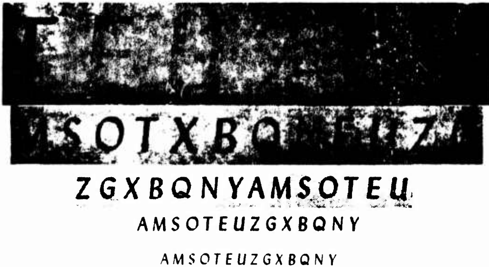
FIGURE 4.1-13. SIZE VERSUS CONTRAST TO YIELD CONSTANT READABILITY (32)
