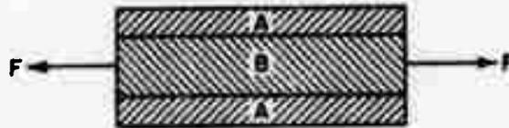
Figure 3. Simplified model for a specimen containing uniform compressive and tensile stresses. Region A is in tension. Region B is in compression.
