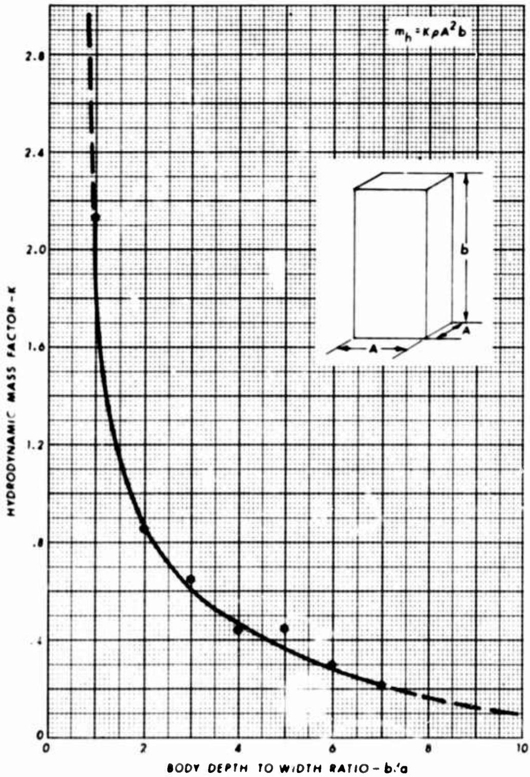
Fig. 12 - Effect of Body Depth to Width Ratio on Hydrodynamic Mass for Vertical Translation of Parallelepipeds
