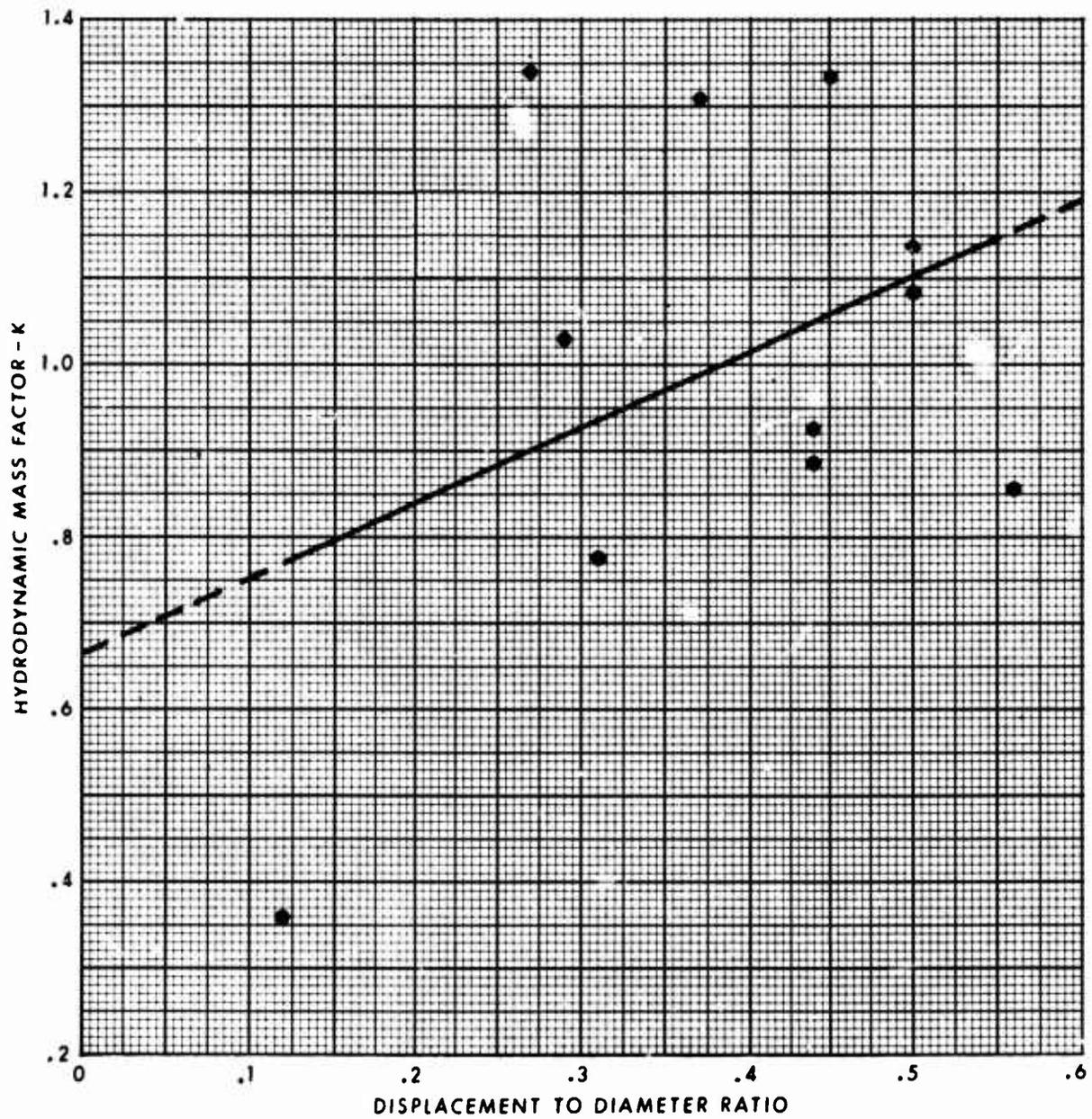
Fig. 7 - Least Mean Squares Plot of Hydrodynamic Mass Factor versus Displacement-to-Diameter Ratio for a 2:1 Ellipsoid with 20% "Wings"
