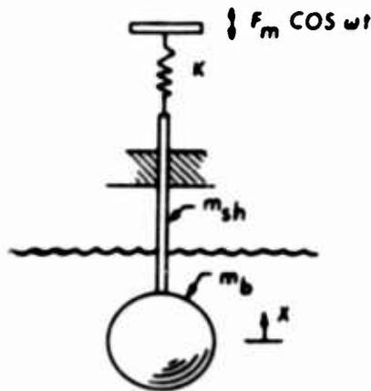
The equation of motion for the system when the body is immersed is:
