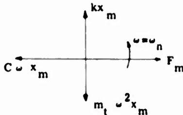
At resonance, the driving force,  $F_m$ , balances the frictional force,  $C \omega x_m$ , and the inertia force,  $m_t \omega^2 x_m$ , balances the spring force,  $kx_m$ . Thus the hydrodynamic mass can be determined by measuring the spring constant, the natural frequency with the body immersed, and the in vacuo mass of the system. Hence,
