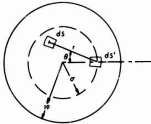
Let  $dp$  be the increment increase in pressure that the motion of  $dS$  produces in the medium at a point adjacent to some other element of area of the piston,  $dS'$ . The total increase in pressure in the medium adjacent to  $dS'$  can be found by integrating
