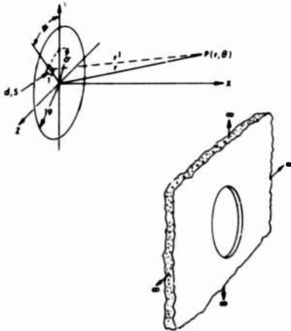
Assume that the piston is moving with simple harmonic motion. The pressure produced at any point by the piston is the sum of the pressures that would be produced at the point by an equivalent assembly of simple sources.
