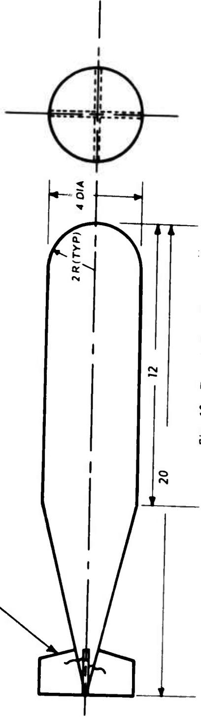
Fig. 16 - Torpedo Body (Body No. 25)
