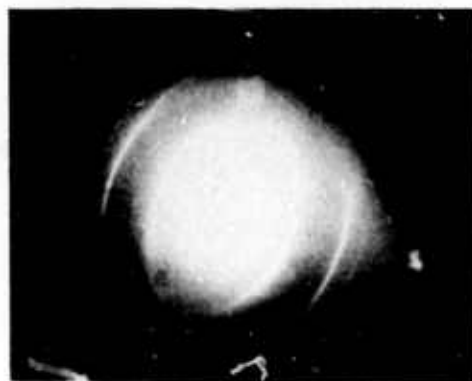
Figure 3b. SAED from 321-31C(2300). Elliptical diffraction pattern characteristic of oriented texture. (002) planes are inclined at an angle of 20 degrees from the beam.
