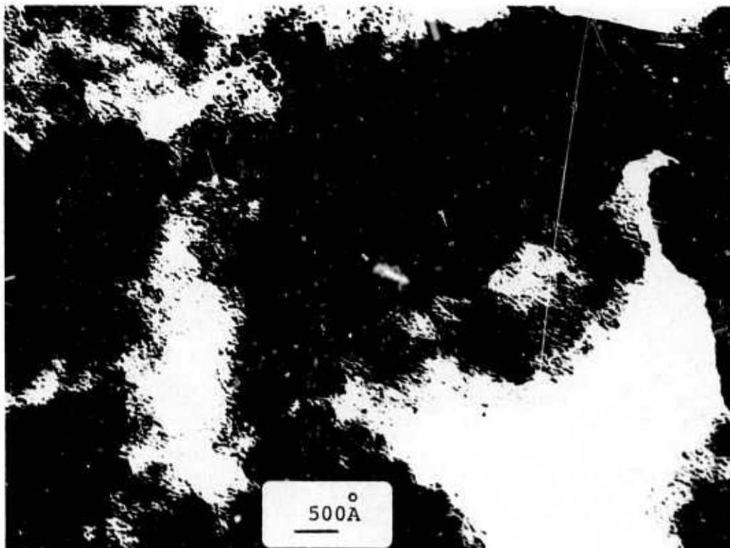
Figure 1a. Sample 321-31D(2300). Typical granular texture characteristic of bulk of the material. The platelets are not very distinct.
