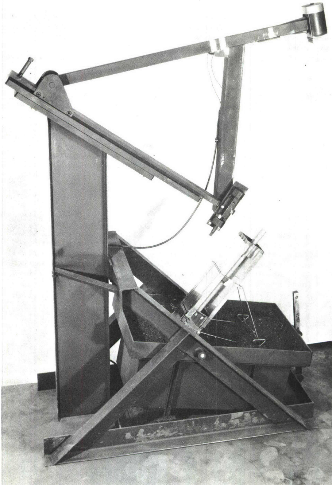
Fig. 4 MODEL OF PENDULUM TEST FIXTURE
