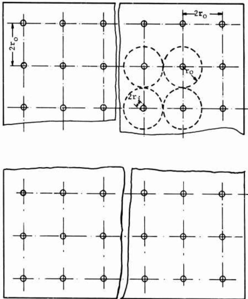
Figure 1. Cross-section of square prism matrix of pipes in an earth heat sink.
