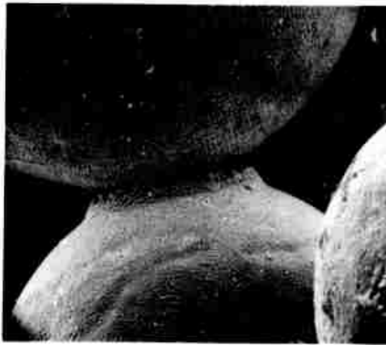
Figure 3 - The formation of interparticle necks from sintering, at 2150°F, in vacuum, of IN 100 powder. 240X.
