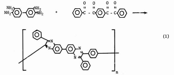
This material possesses superior thermal properties and is easily processed into usable forms. Its chief drawback is its expense which results from the high cost of the p-bis(phenylglyoxaloyl)benzene used in its preparation. This is due to the rather complex synthetic route currently used to produce the material.<sup>2</sup> We, therefore, sought to eliminate this drawback by devising a more efficient, less costly synthesis of this compound. Such a synthesis is the subject of this report.
