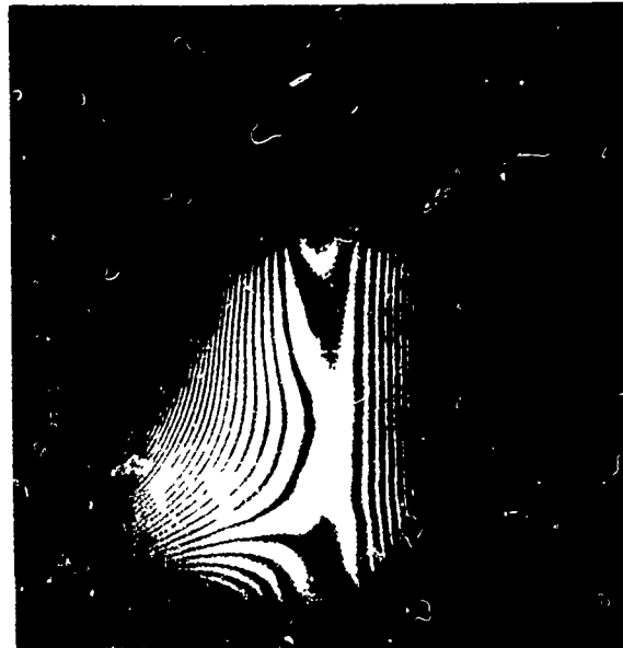
(b) BEAM EXPANSION WITH DIFFUSER PLATE
