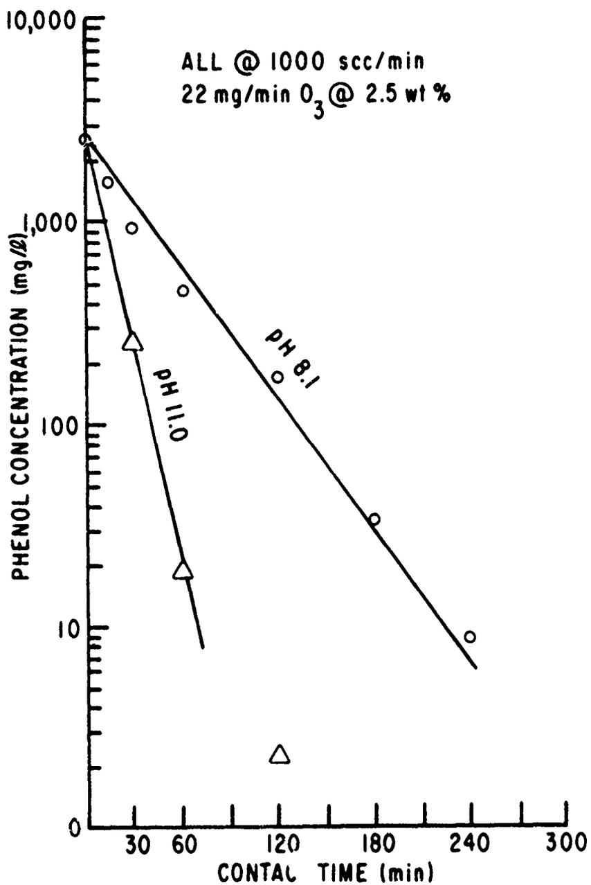
Figure 9. Phenol Concentration Versus Batch Contact Time for Varying pH
