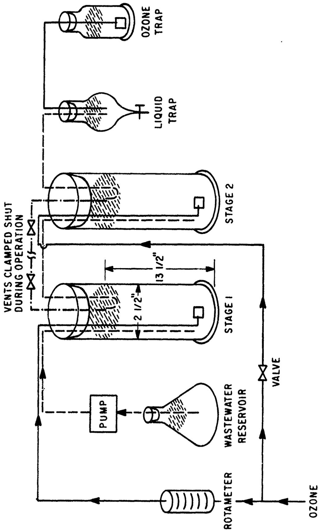
Figure 7. Continuous Flow Apparatus for Ozonation Experiments
