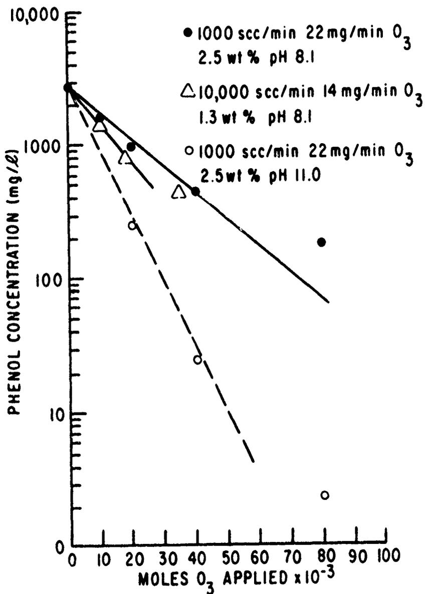
Figure 11. Phenol Concentration Versus Moles Ozone Applied (Batch)
