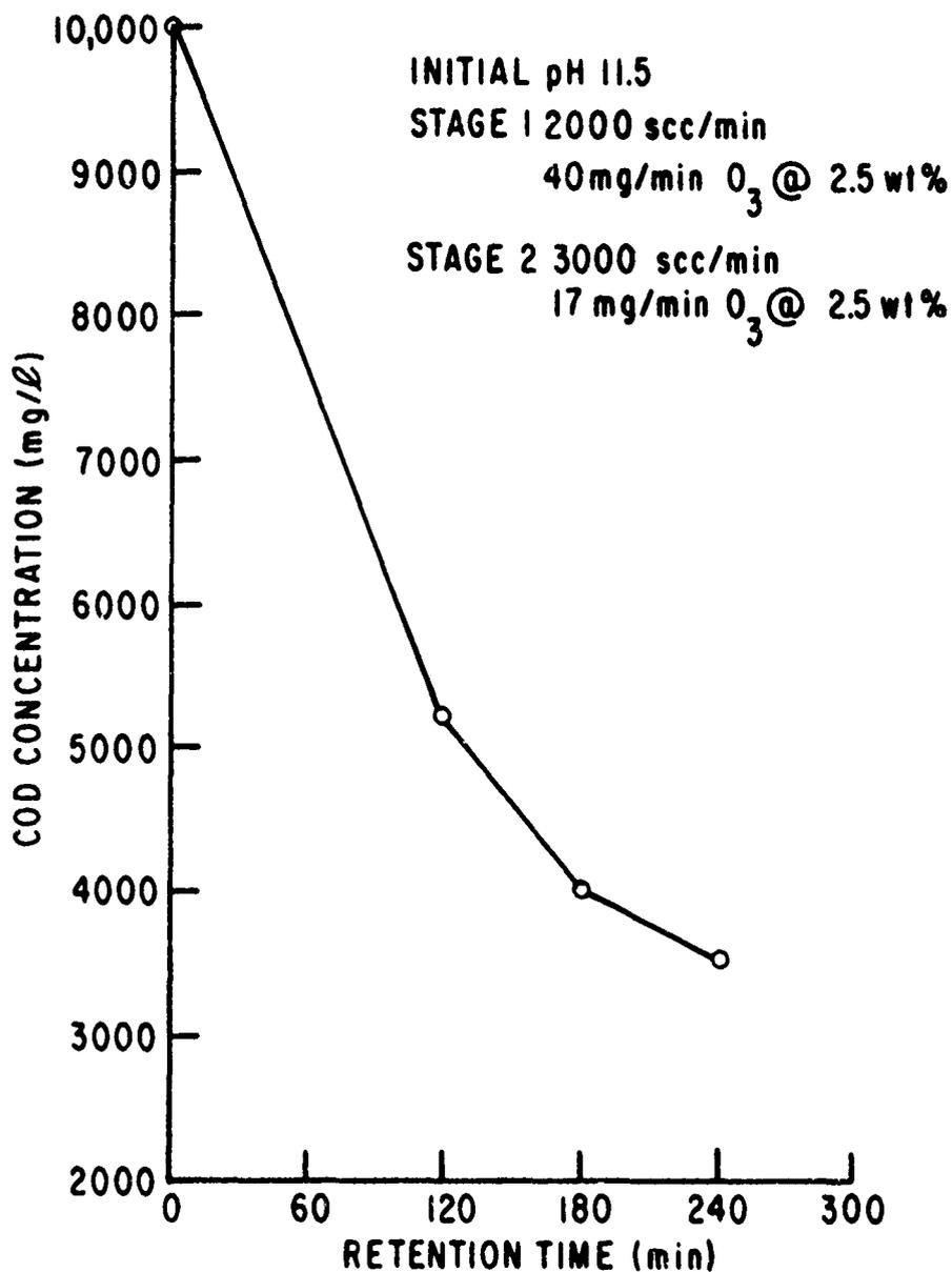
Figure 17. COD Concentration Versus Continuous Flow Retention Time
