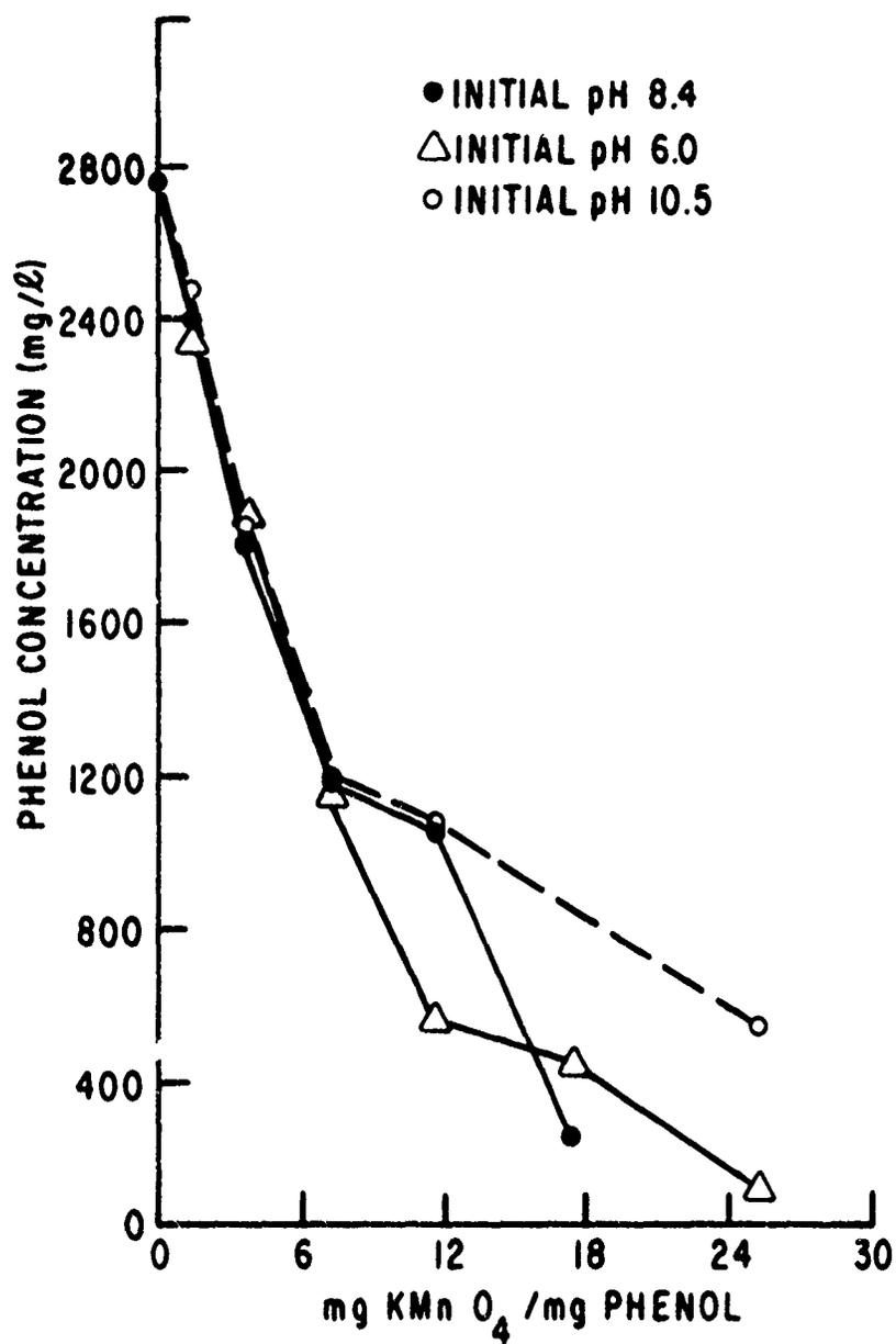
Figure 19. Phenol Concentration Versus mg  $KMnO_4$  Applied/mg Phenol
