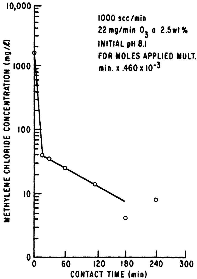
Figure 13. Methylene Chloride Concentration Versus Batch Contact Time
