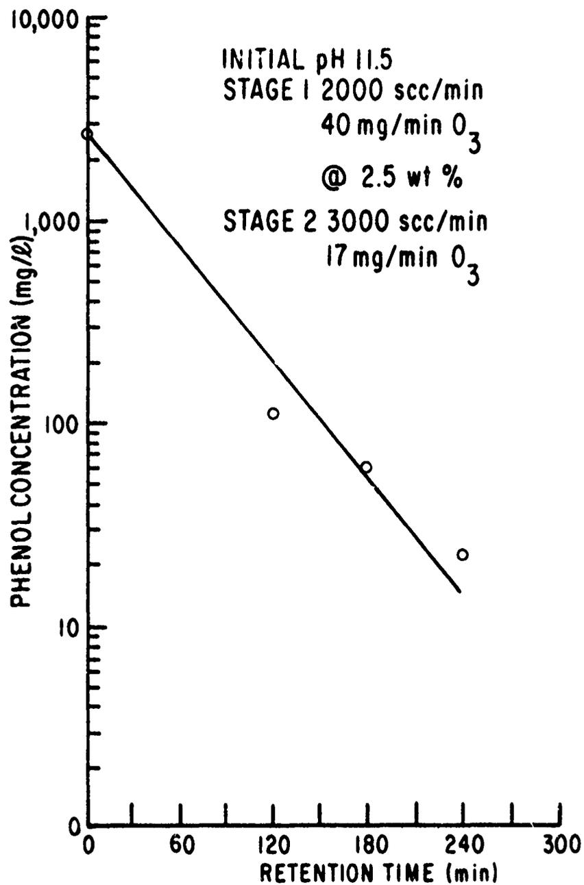
Figure 16. Phenol Concentration Versus Continuous Flow Retention Time
