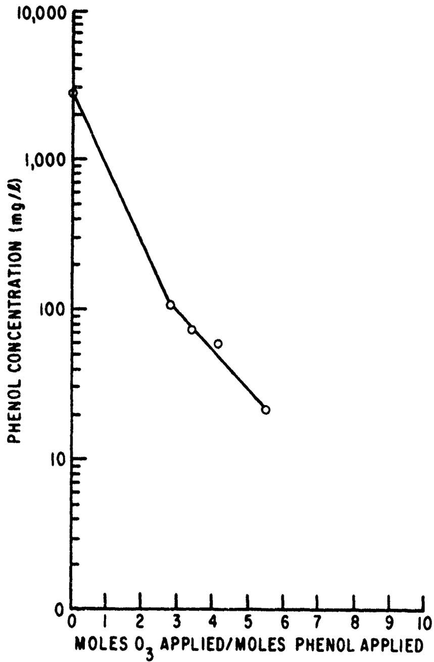
Figure 18. Phenol Concentration Versus Moles O<sub>3</sub> Applied/Moles Phenol Applied
