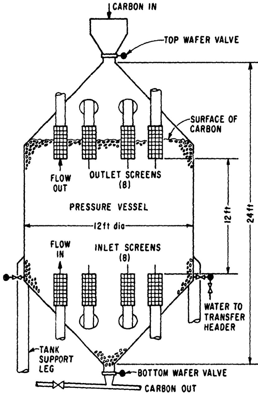
Figure 5. Section Through Activated Carbon Column
