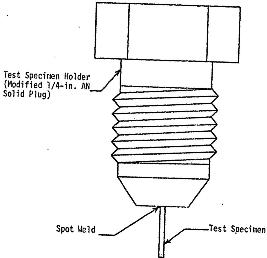
Figure 13. Schematic of Test Specimen Holder with Test Specimen in Place.
