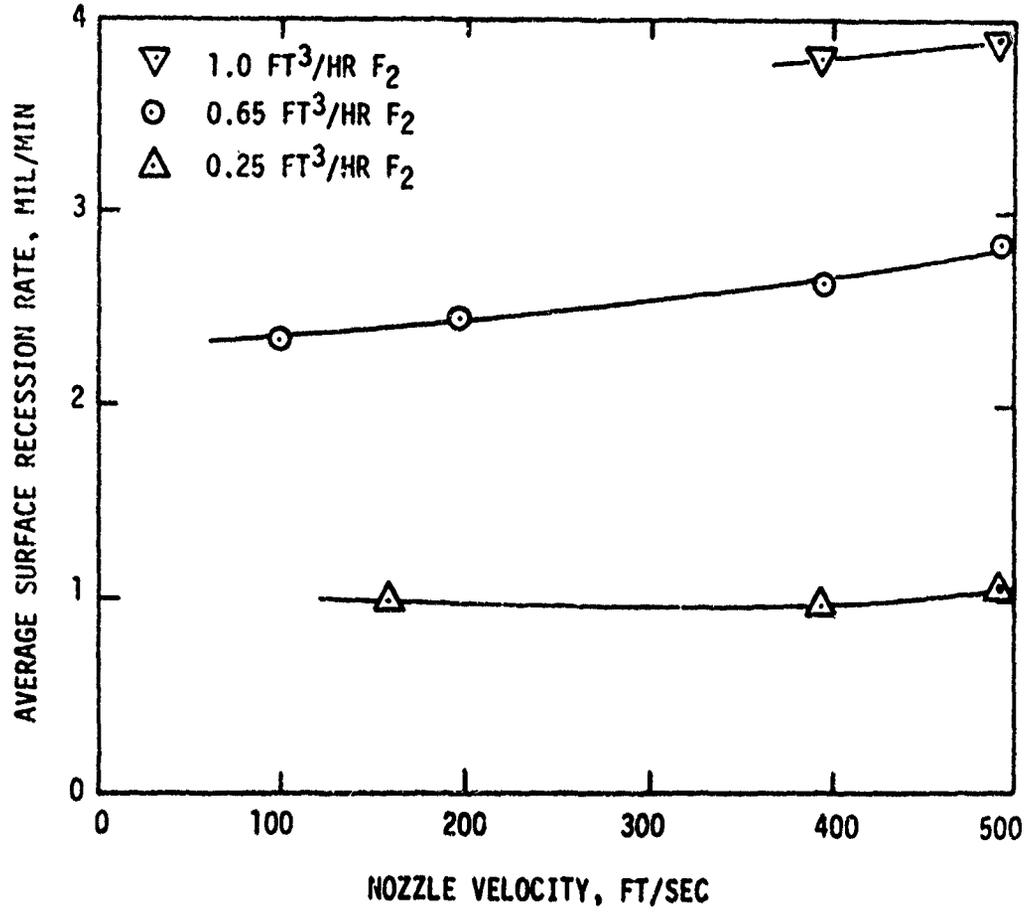
Figure 4. Effect of Nozzle Velocity on the Corrosion Rate of Tungsten at 4000°F and a Nozzle Distance of 1 in.
