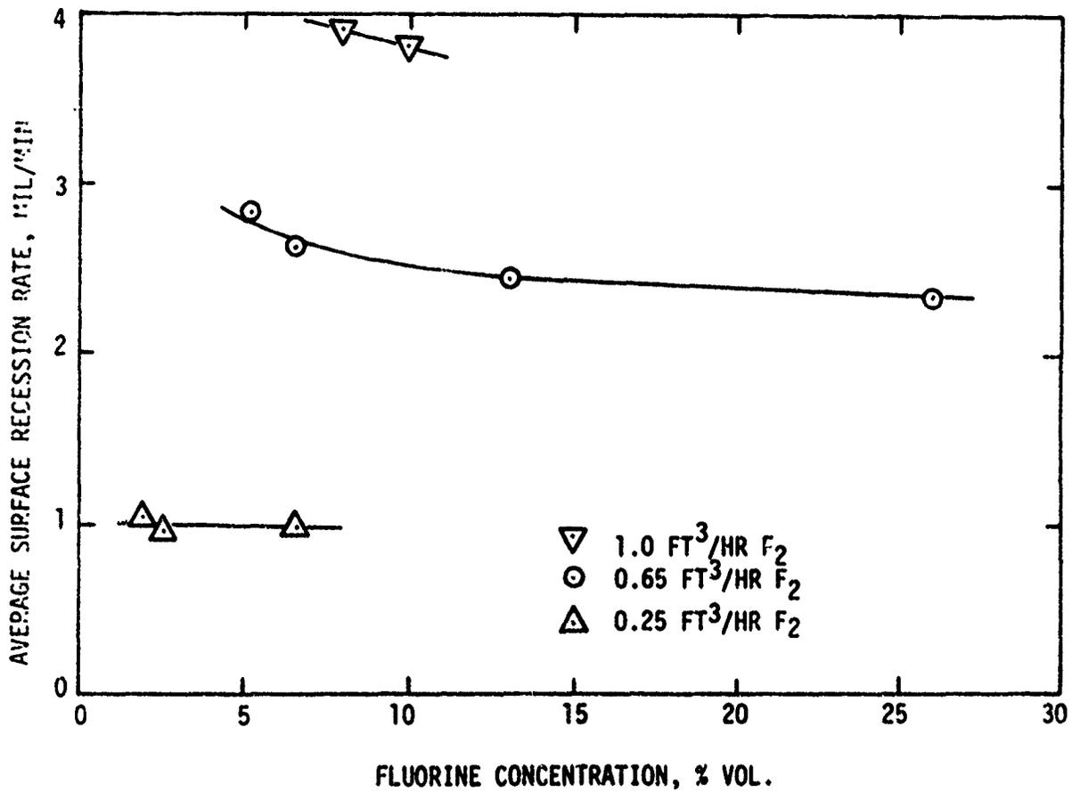
Figure 5. Effect of Fluorine Concentration on the Corrosion Rate of Tungsten at 4000°F and a Nozzle Distance of 1 in.
