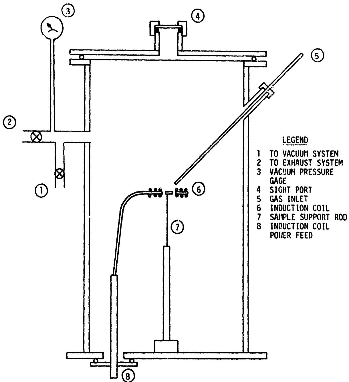
Figure 1. Schematic Diagram of Refractory Metals/Fluorine Reaction Chamber
