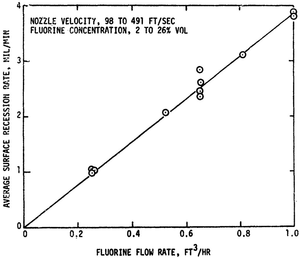
Figure 3. Effect of Fluorine Flow Rate on the Corrosion Rate of Tungsten at 4000°F and a Nozzle Distance of 1 in.
