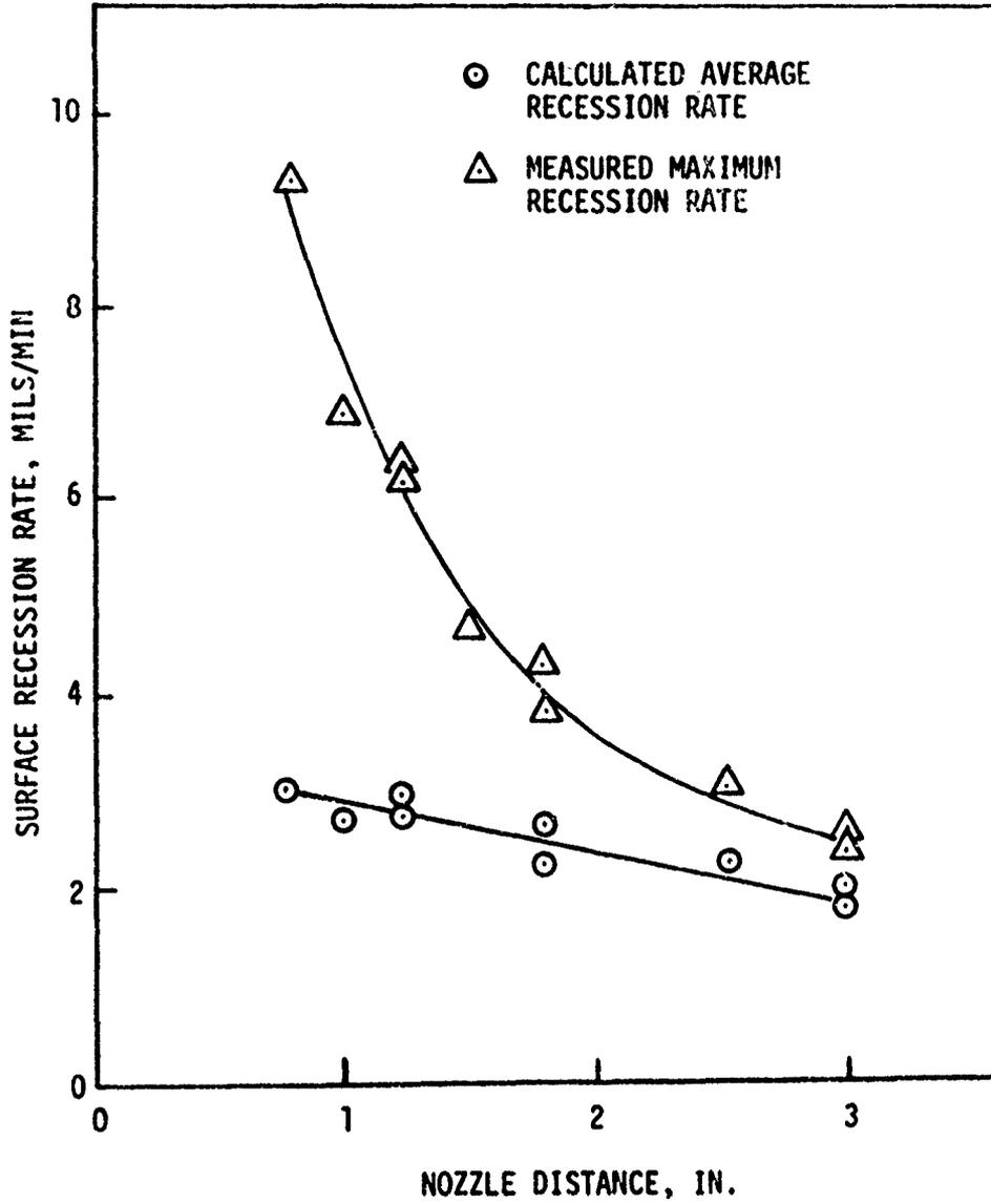
Figure 2. Effect of Nozzle Distance on the Corrosion Rate of Tungsten at 4000°F in Fluorine-Argon Mixture (6.5/93.5 vol)
