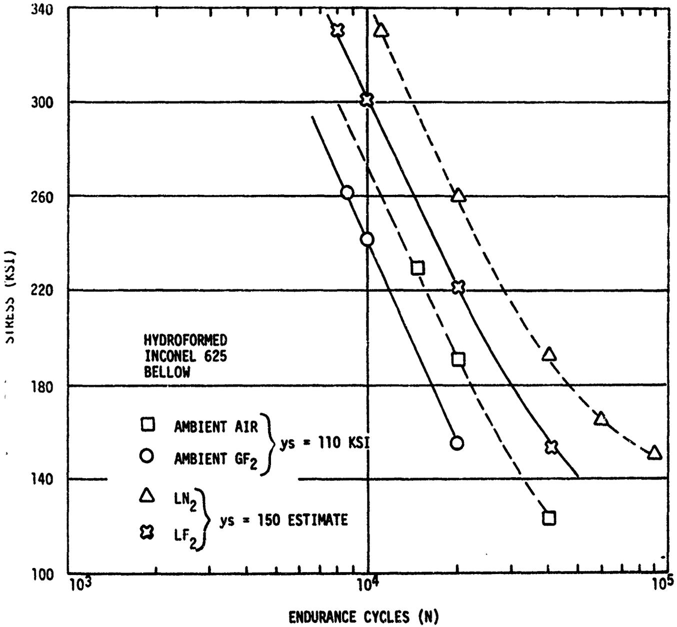
Figure 9. Fatigue Strength of Hydroformed Inconel 625 Bellows in Fluorine Environments
