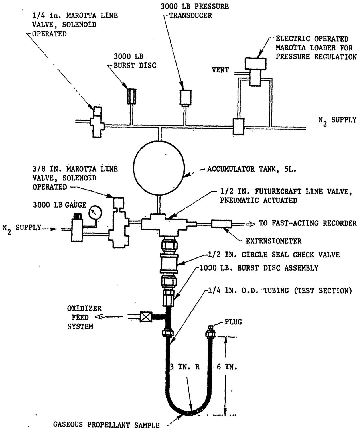
Figure 11. Schematic Diagram of U-tube Adiabatic Compression Apparatus
