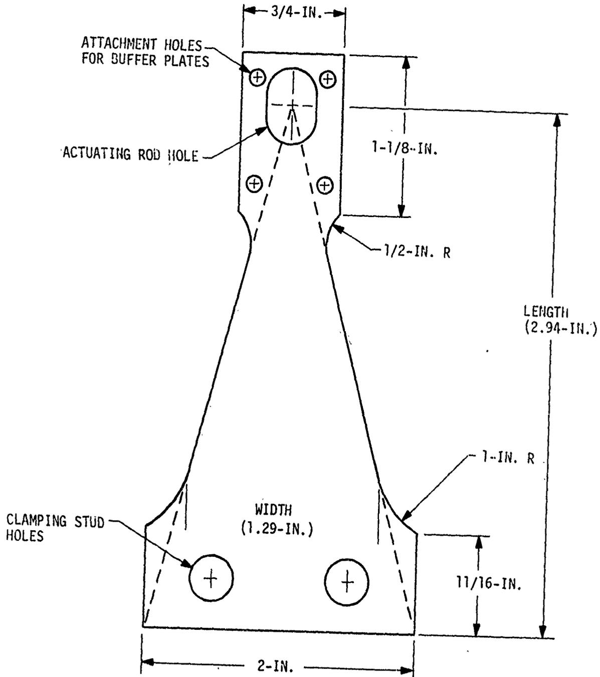
Figure 28. Flexure Test Specimen
