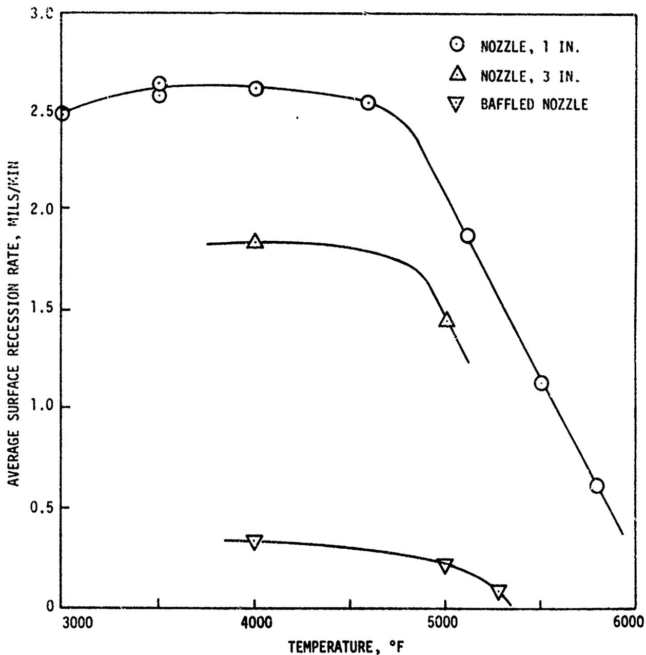
Figure 6. Effect of Temperature and Flow Conditions on the Corrosion Rates of Tungsten in a Fluorine-Argon Gas Mixture (6.5/93.5 vol)
