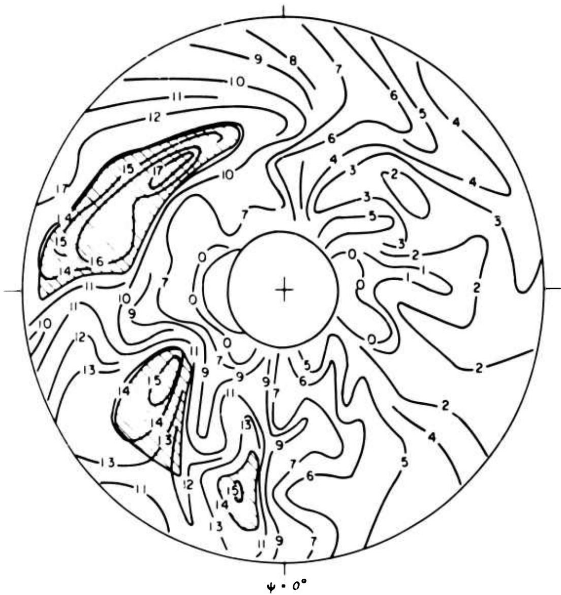
Fig 17 Blade angle of attack distribution for case of Figure 15: \mu = 294 , \tau = 0^\circ , \frac{c_1}{\sigma} = 0.11
