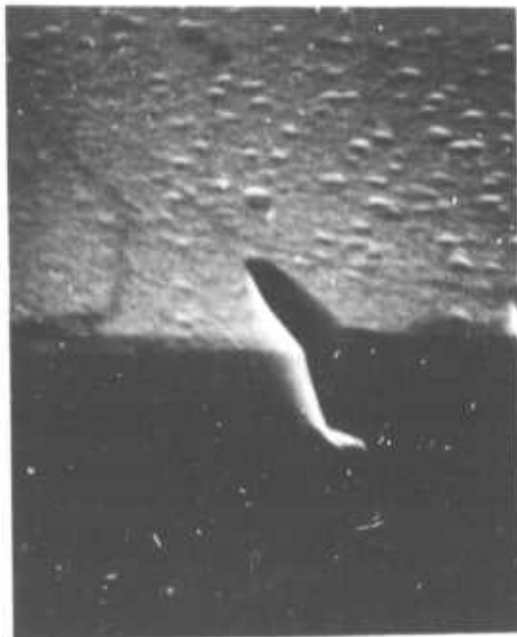
Fig. 10. SEM micrographs of split. (a) From etch figures corresponding to Fig. 9. (b) Cross section of two different splits.
