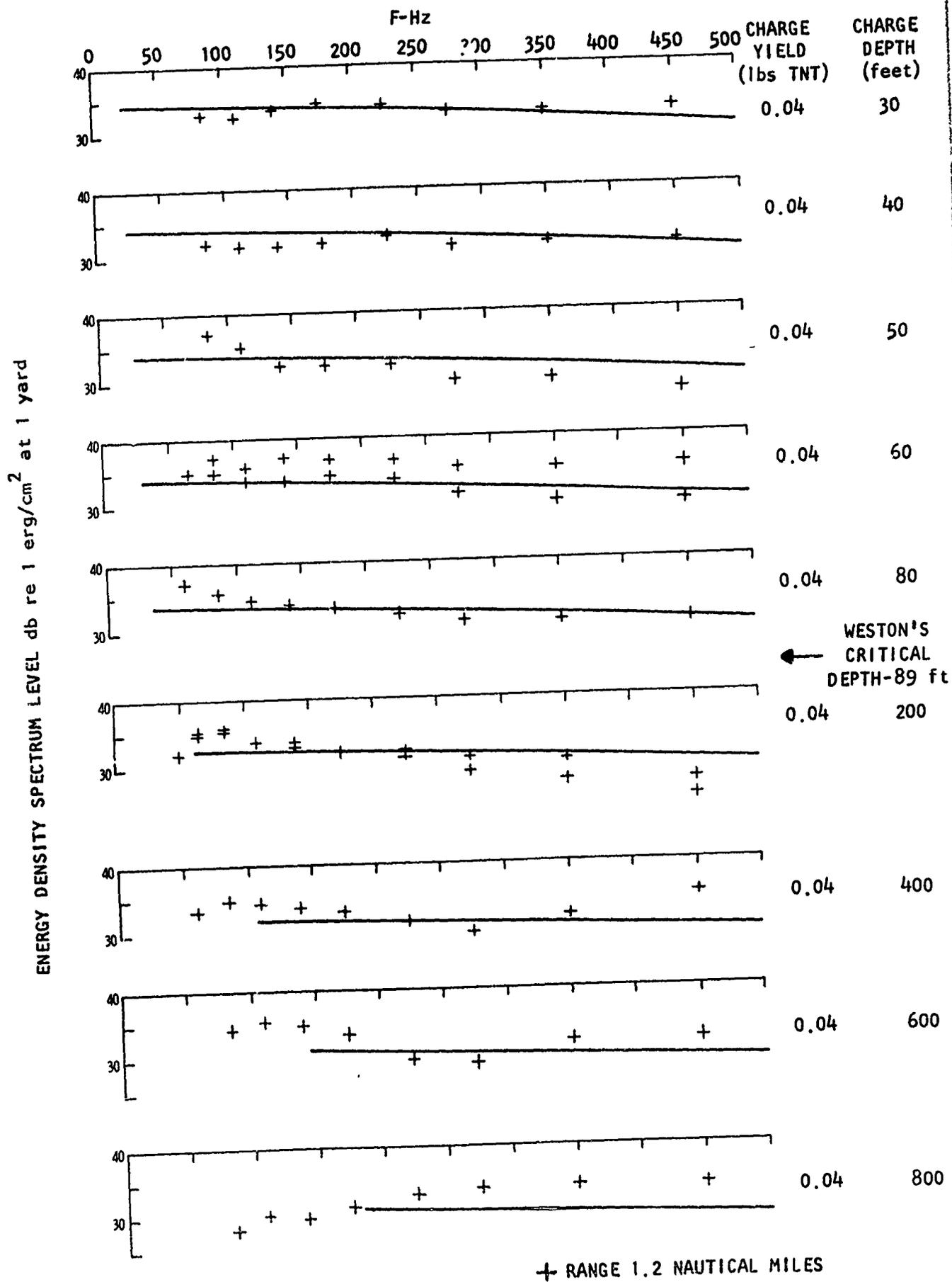
Figure 5. Measured Source Level and Weston's Predicted Source Level 13
