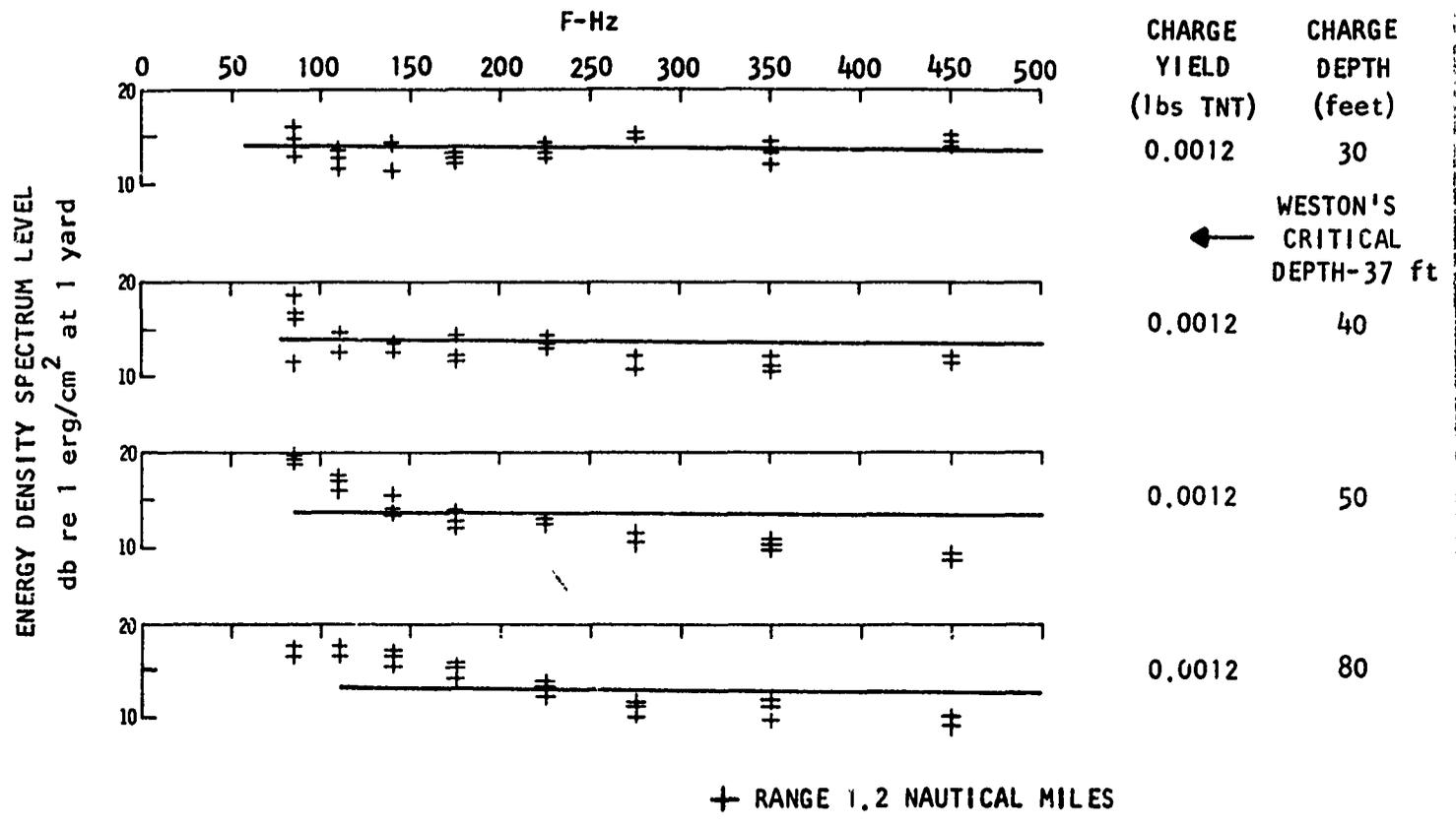
Figure 4. Measured Source Level and Weston's Predicted Source Level
