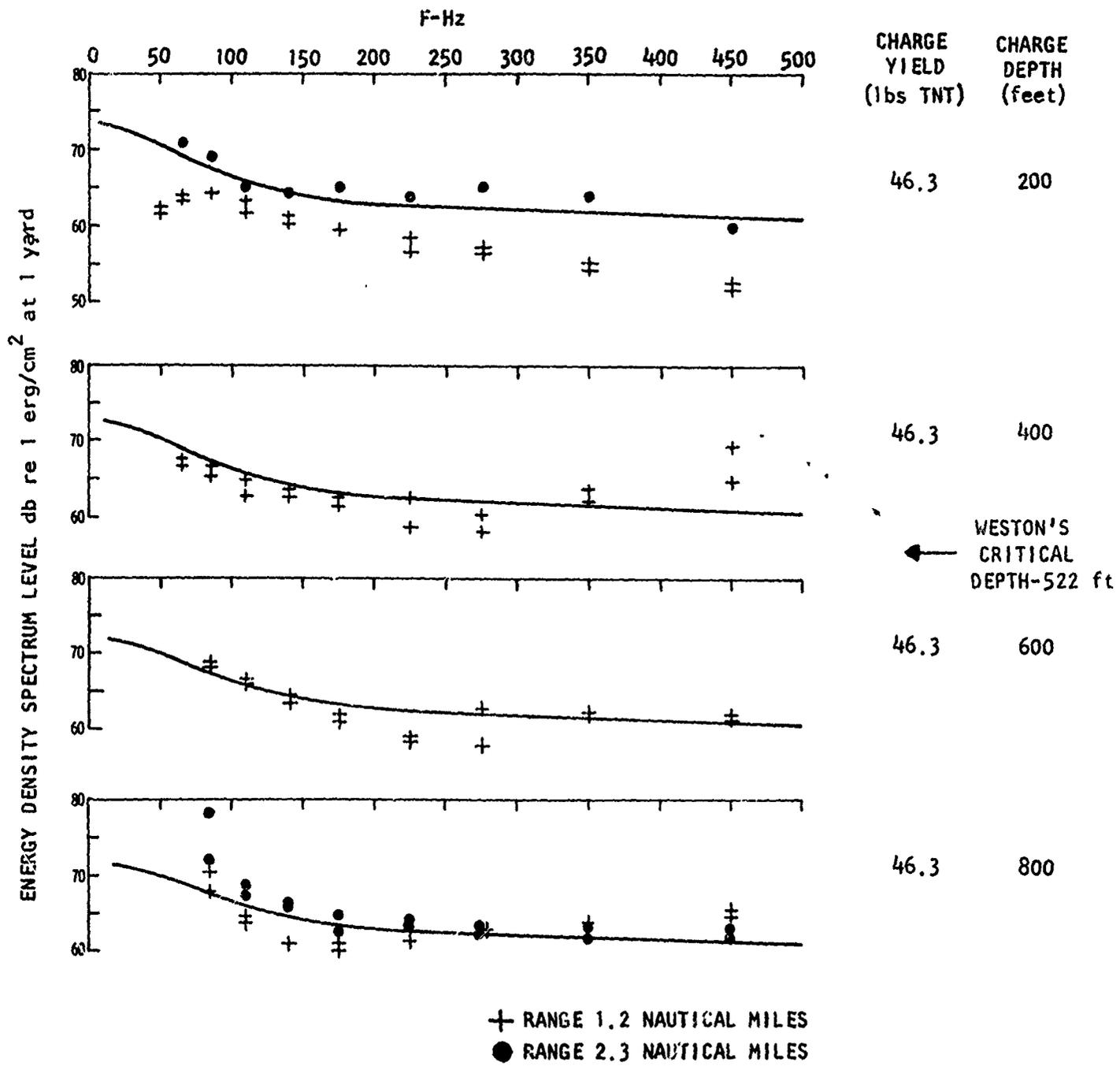
Figure 8. Measured Source Level and Weston's Predicted Source Level
