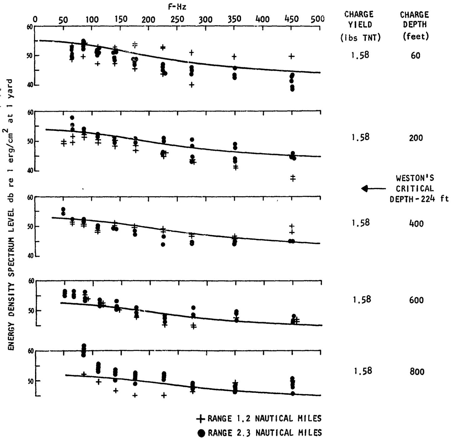
Figure 7. Measured Source Level and Weston's Predicted Source Level
