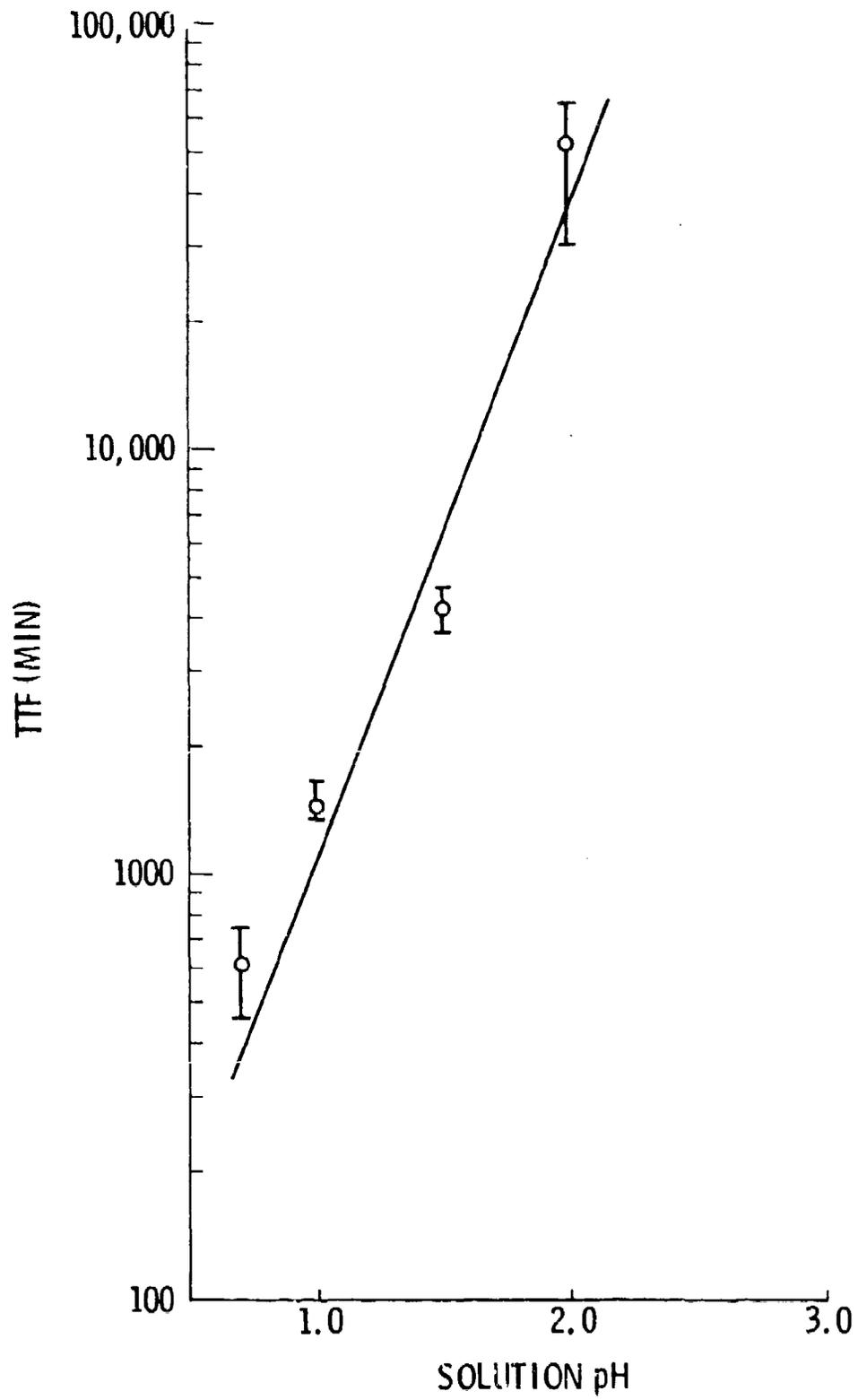
Fig. 3 Log TTF Versus pH for -T7351 AR
