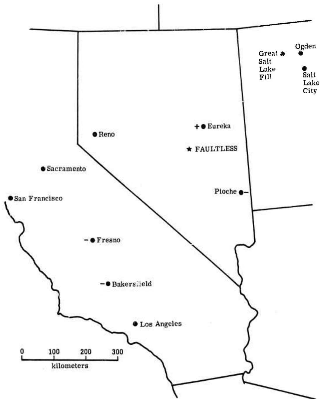
FIGURE 7. FIRST-ZONE SEISMIC STATIONS FOR FAULTLESS. Any plus and minus signs indicate P-wave first-motion polarity.
