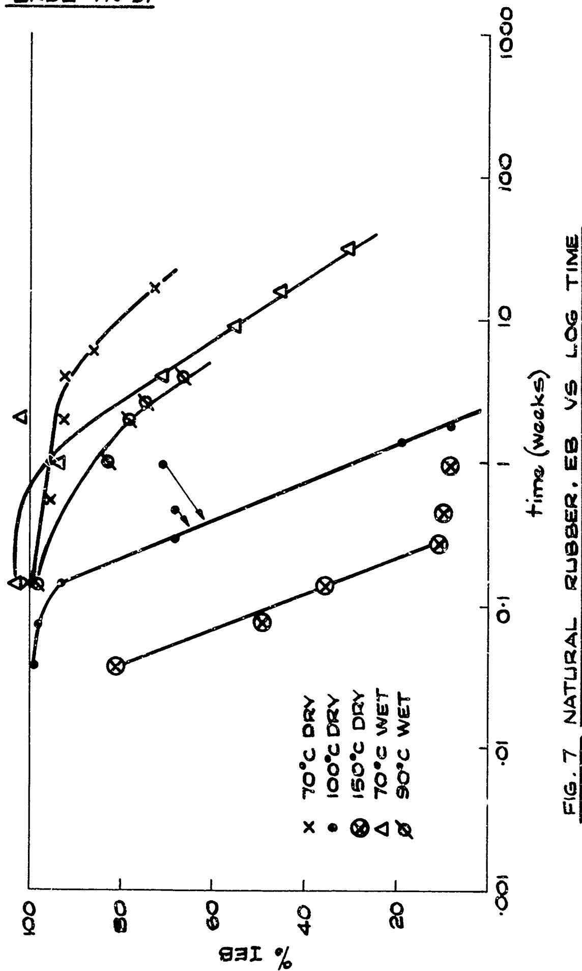
FIG. 7 NATURAL RUBBER. EB VS LOG TIME
