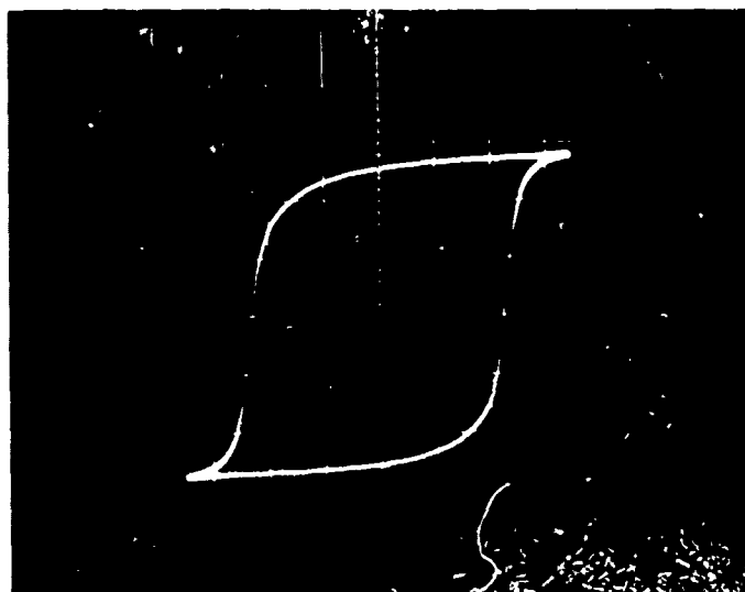
Figure 7 Hysteresis loop observed on latest Honeywell coarse-grained ceramics. Scale: vertical, 20 \mu\text{C}/\text{cm}^2 and horizontal, 2.35 \text{ KV}/\text{cm} .
