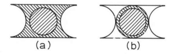
Figure 1. Cross Section of Double-U Laser Rod Configurations (a) Active cylindrical core with "double-U" cladding uniformly doped with Nd<sub>2</sub>C<sub>3</sub> and Yb<sub>2</sub>O<sub>3</sub> to provide both sensitizing cladding and optical coupling.
