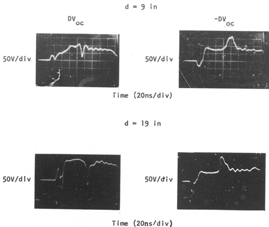
Figure 6. Differential open circuit voltage at the terminals of a two-wire transmission line (poor common mode rejection).
