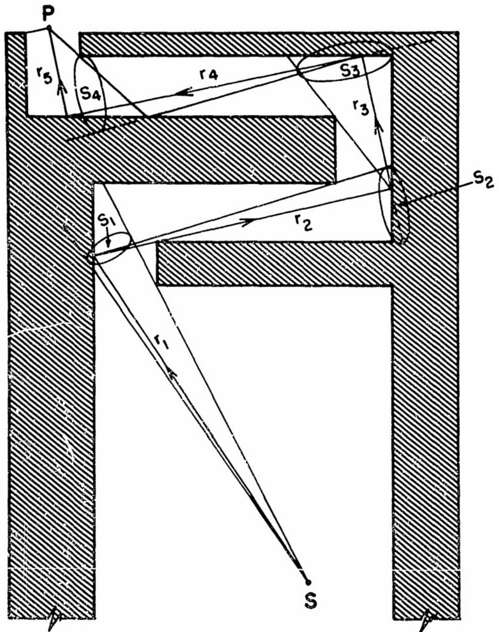
Figure VII-3 - Example 2 labyrinth for calculation
