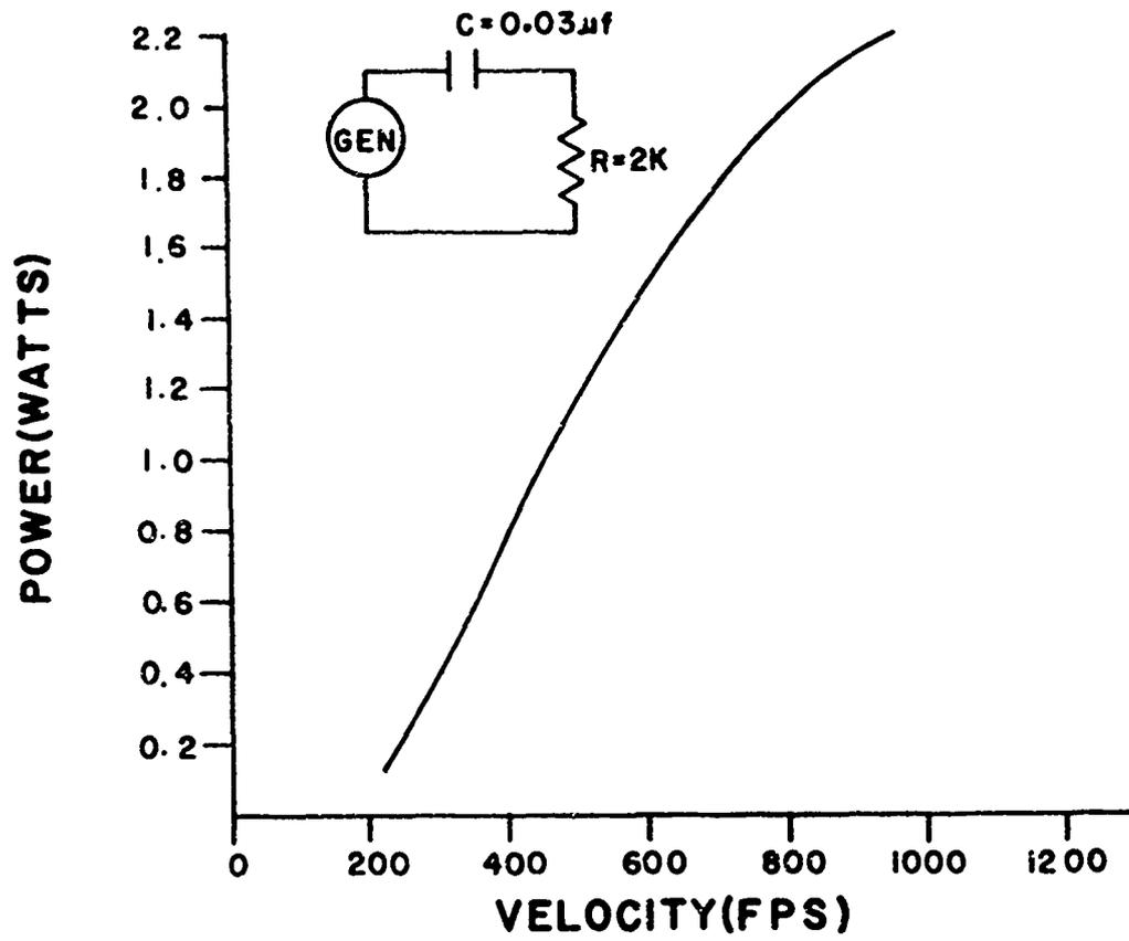
Figure 14. Electrical output of E-frame fluidic generator.
