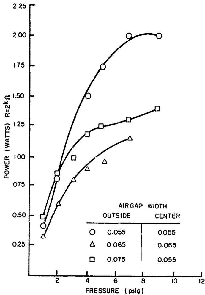
Figure 11. Effects of airgap sizes versus output power.
