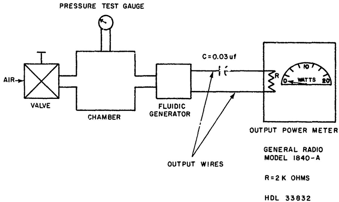
Figure 6. Laboratory arrangement of calibrated test equipment.
