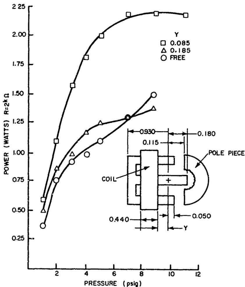
Figure 12. Effects of coil position versus output power.
