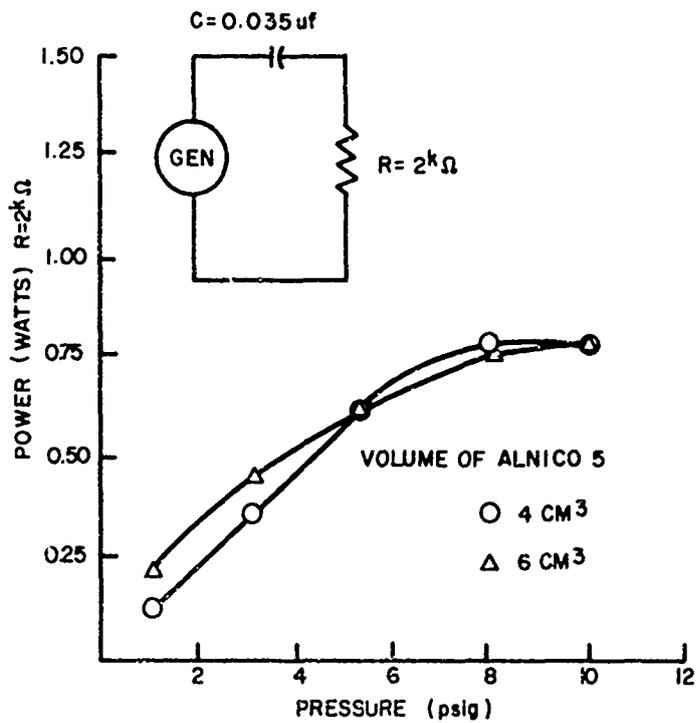
Figure 7. Effects of magnet volume upon output power.
