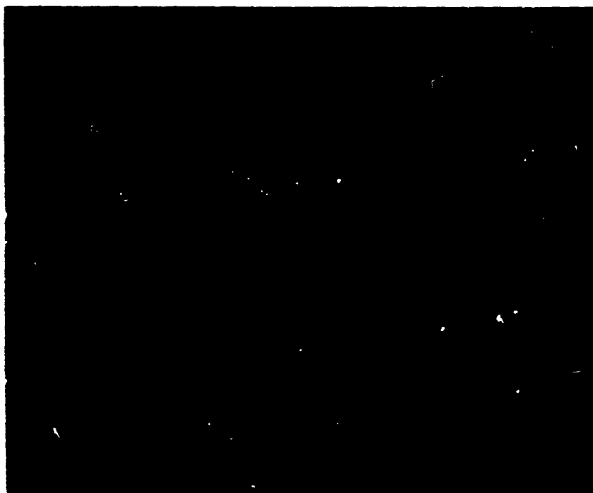
Fig. 13 Ultramicroscope photomicrograph of scattering centers in a NDY ceramic rod. 10X
