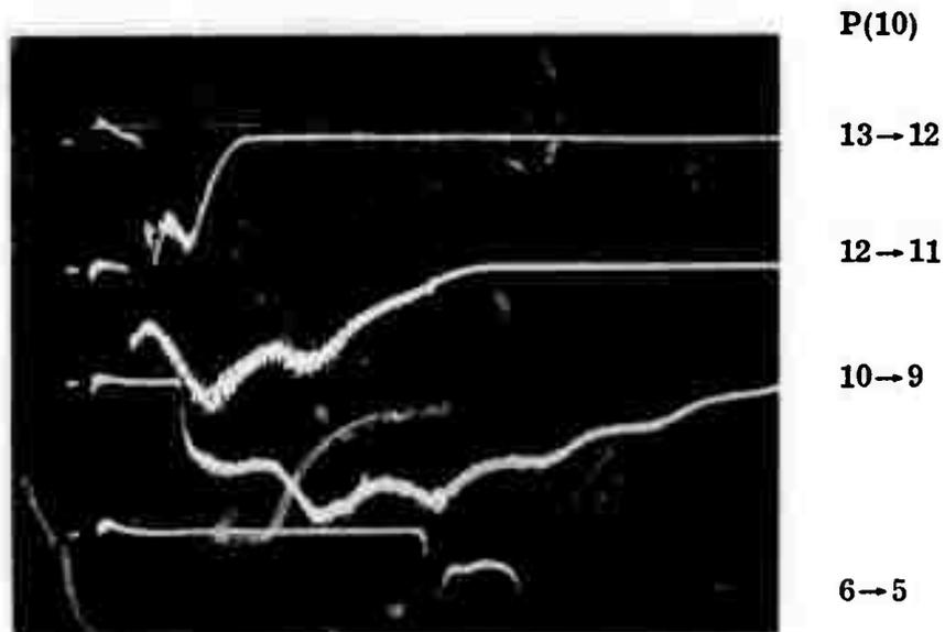
**FIGURE 7.** Change of time delay for initiation of  $P(10)$  laser pulse, as a function of vibrational level (abscissa:  $20\mu\text{s}/\text{div}$ ; ordinate for  $v = 13 \rightarrow 12$  through  $v = 6 \rightarrow 5$  transitions:  $0.01, 0.05, 0.05, 0.02 \text{ v}/\text{div}$ ).
