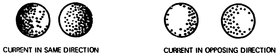
FIGURE 11-2 PROXIMITY EFFECT OF CURRENT IN TWO PARALLEL WIRES
