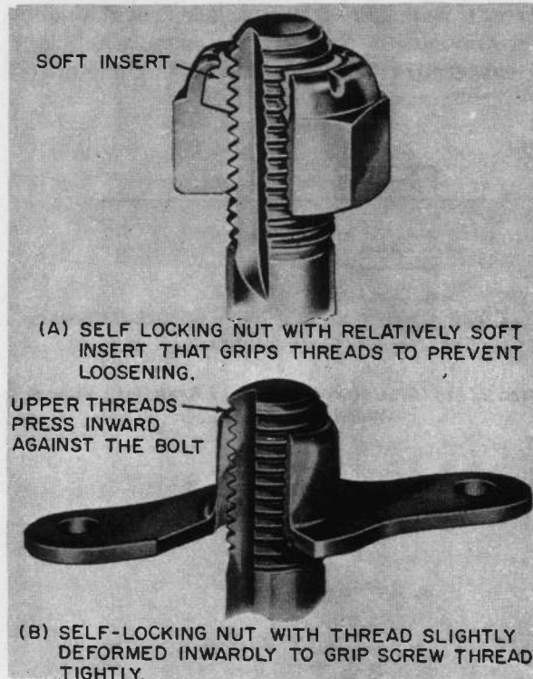
Figure 21-17. Self-Locking Nuts (Courtesy of Elastic Stop Nut Corp.)
