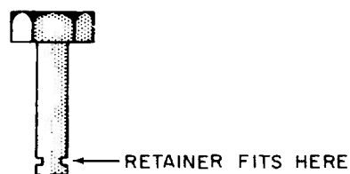
figure 21-24. Specially Designed Bolts Used With Retainer Rings
