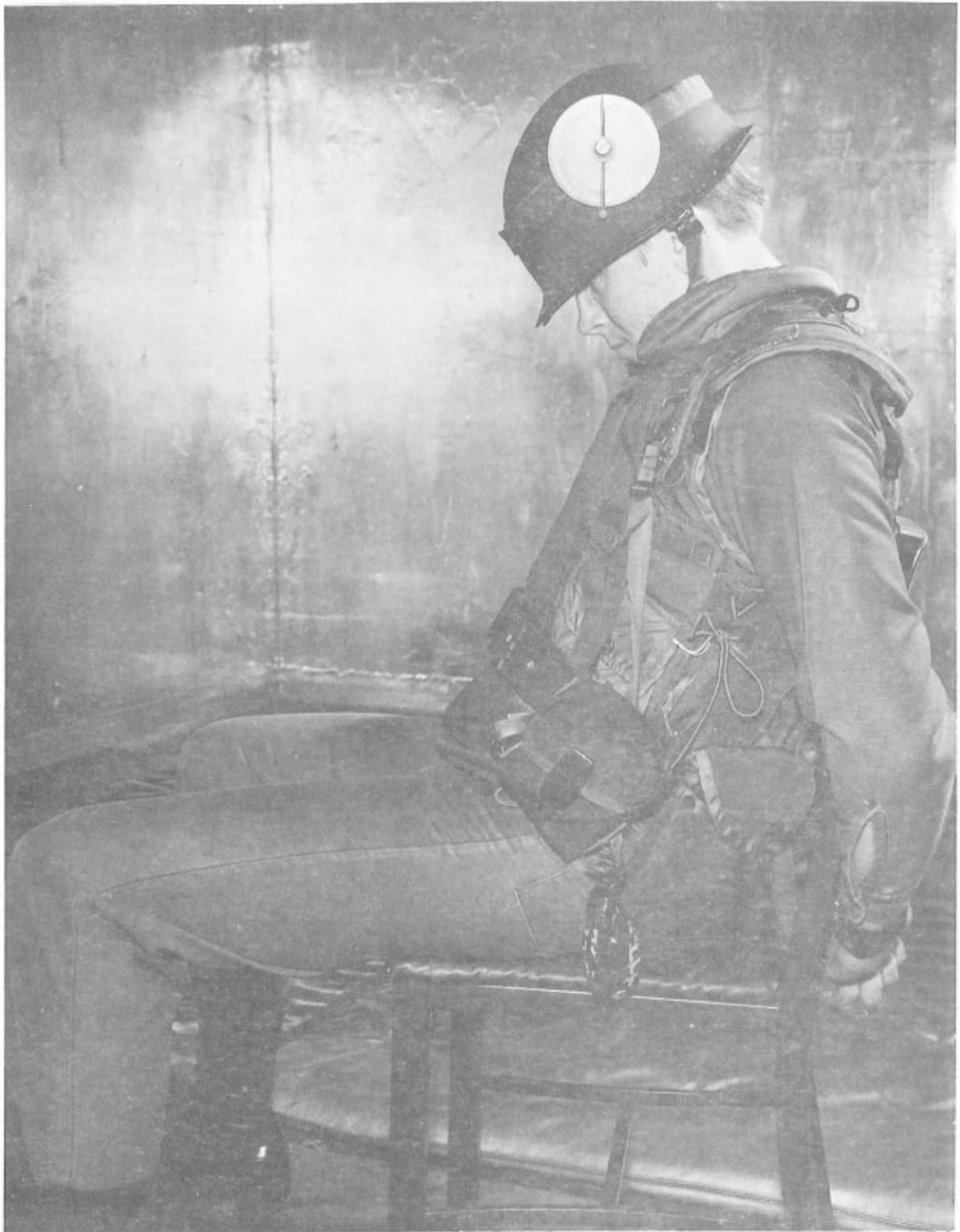
Figure 2. Head Movement Ventral to Dorsal. Goniometer set to zero with head in ventral position.
