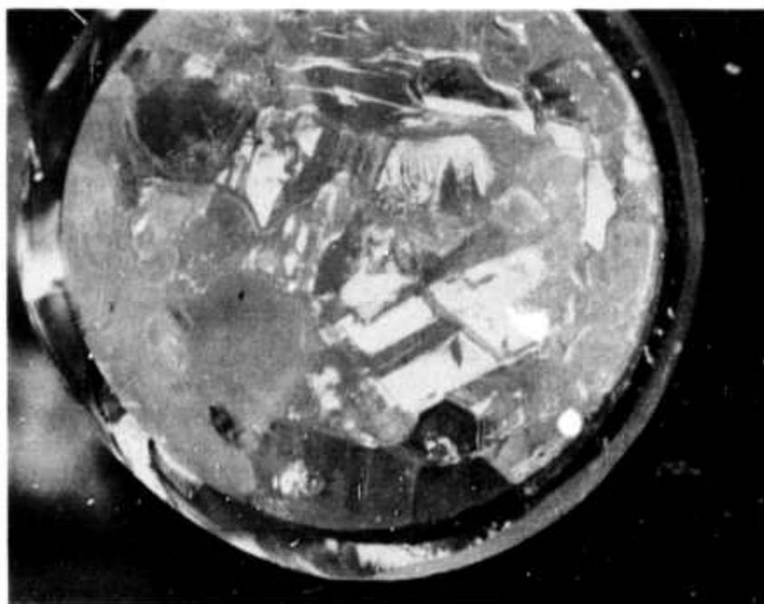
Figure 19 The concave interface of growing salol containing many large facets (30 mm OD tube, BSA-7A).
