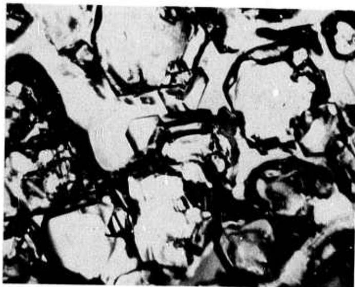
Figure 25 Surfaces of solidified naphthalene at tube wall.
