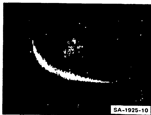
FIGURE 7 TIME HISTORY OF MOLECULAR RADIATION AT 4570\text{\AA} (PRESSURE = 5400 torr, 1\text{ }\mu\text{sec/cm} )
