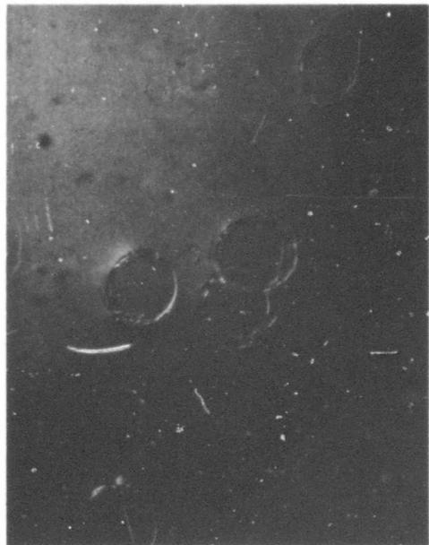
FIGURE 13 RING FRACTURES ON THE SURFACE OF SPECIMEN G2
