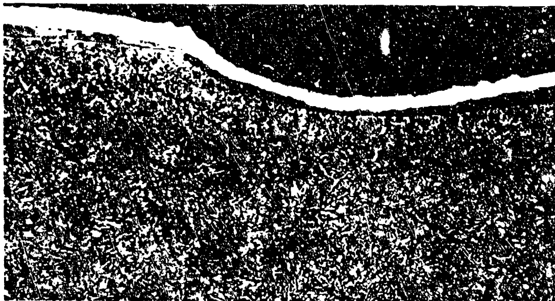
FIGURE 8 PHOTOMICROGRAPH REVEALING THE TRANSVERSE STRUCTURE ALONG THE BORE SURFACE OF AN UNPLATED RIFLED INSERT AFTER 5 VENTED BOMB SHOTS WITH WC846 PROPELLANT.
