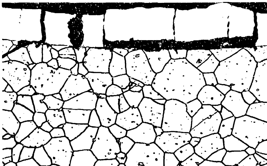
FIGURE 74 TRANSVERSE SECTION AT 1 1/2 INCHES FROM THE CHAMBER OF A CHROME-PLATED CG-27 ALLOY BARREL AFTER FIRING 4,036 ROUNDS AND BEING DECLARED UNSERVICEABLE.
