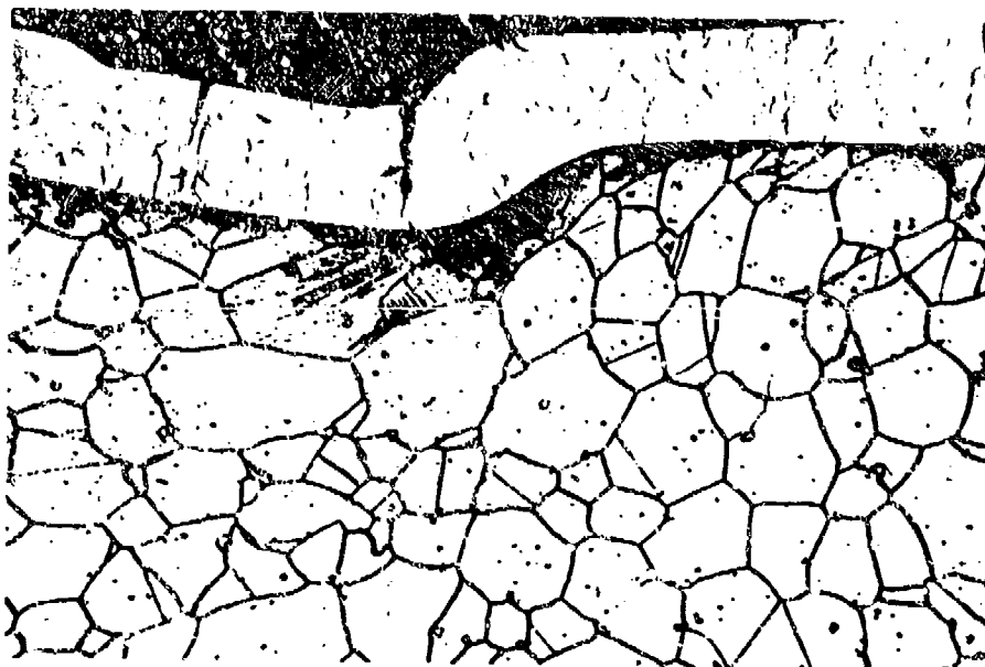
FIGURE 83 TRANSVERSE SECTION AT 17 1/2 INCHES FROM THE CHAMBER OF A CHROME-PLATED CG-27 ALLOY BARREL AFTER FIRING 7,324 ROUNDS AND BEING DECLARED UNSERVICEABLE.
