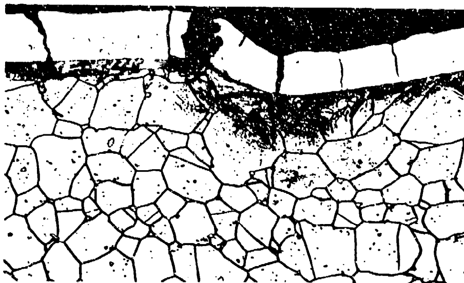
FIGURE 81 TRANSVERSE SECTION AT 2 INCHES FROM THE CHAMBER OF A CHROME-PLATED CG-27 ALLOY BARREL AFTER FIRING 7,324 ROUNDS AND BEING DECLARED UNSERVICEABLE.
