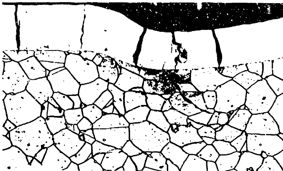
FIGURE 73 TRANSVERSE SECTION AT 1/2 INCH FROM THE CHAMBER OF A CHROME-PLATED CG-27 ALLOY BARREL AFTER FIRING 4,036 ROUNDS AND BEING DECLARED UNSERVICEABLE.
