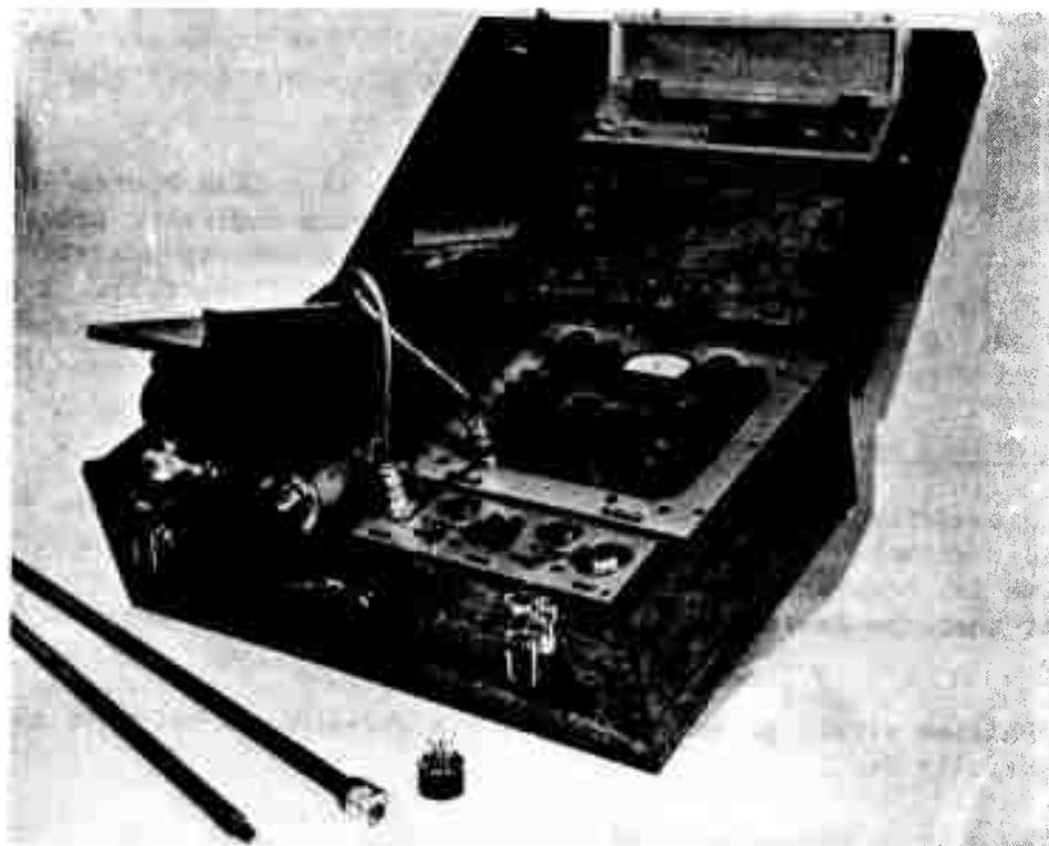
Fig. 11. The control box/carrying case for the doorstopper equipment.
