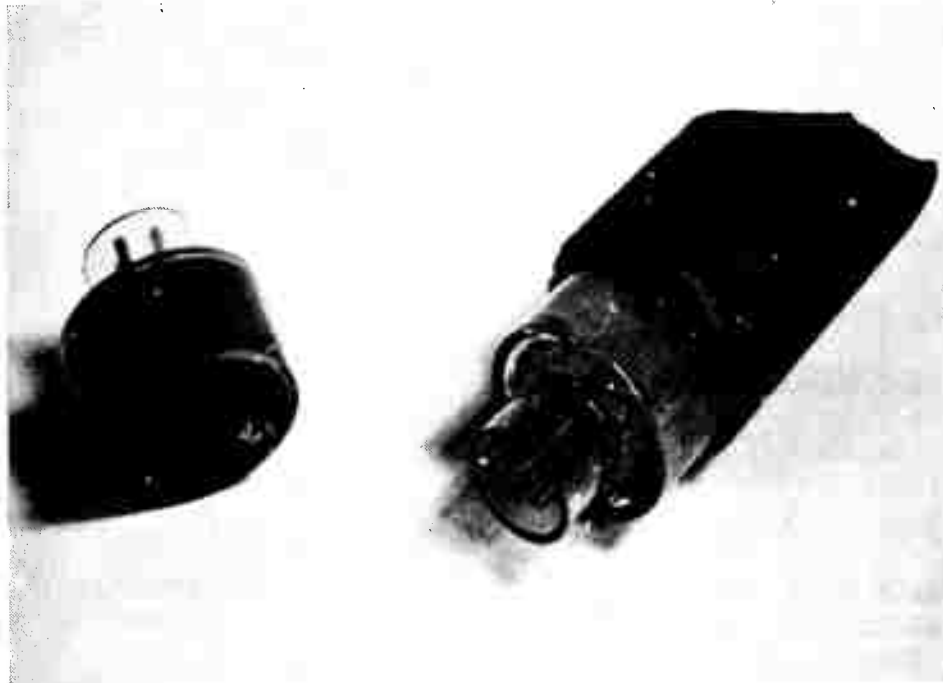
Fig. 8 A doorstopper (left) showing the rosette strain and gauge and and (right) glued to a short length of core.
