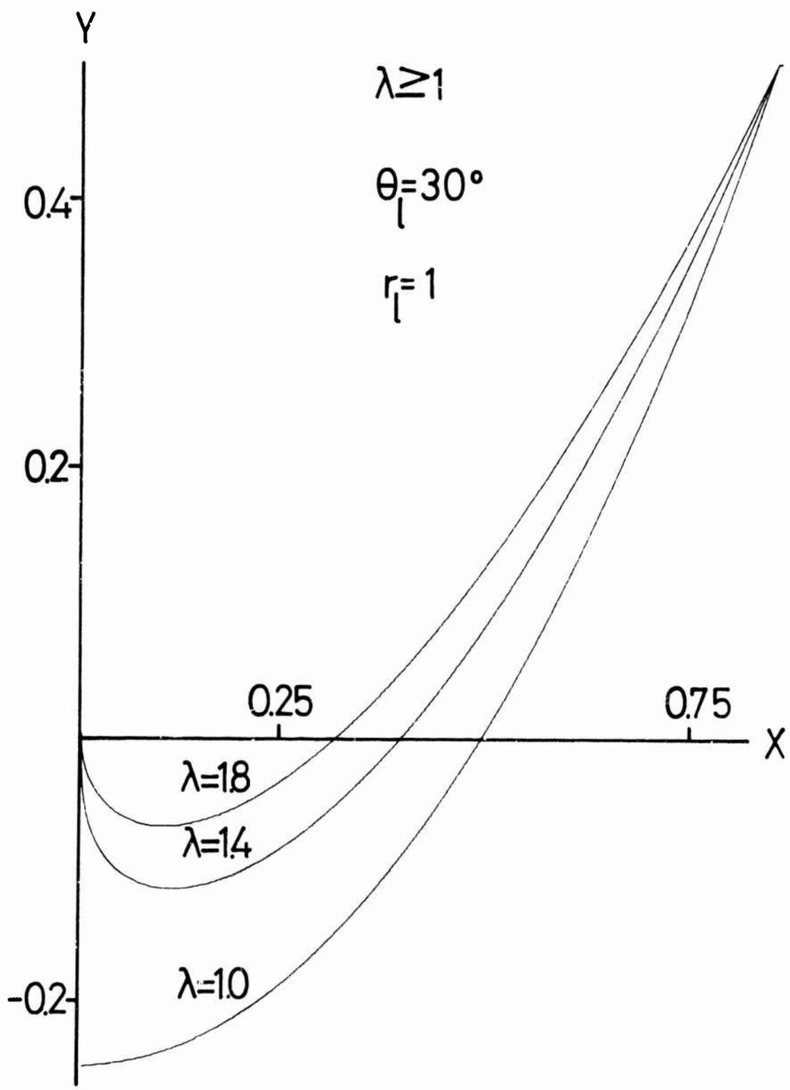
FIGURE 3: RADIAL HOMING TRAJECTORIES WHEN  $\lambda \geq 1$
